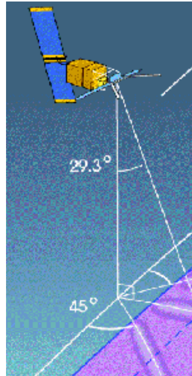
Figure 2. Geometry of the ERS scatterometer showing the three look directions
