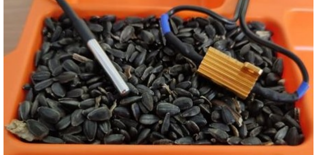
Fig. 4. The first test of hardware for simulating an artificial hot-spot — covered with grain during the duration of the experiment.
