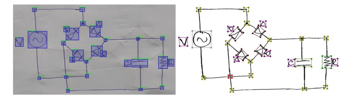
be used for instance segmentation machine learning. Graph structures can trivially be extracted from target values by matching the keypoints ( $\rightarrow$  ports) of electrical symbols ( $\rightarrow$  nodes) geometrically with the keypoints of wire shapes ( $\rightarrow$  edges).
