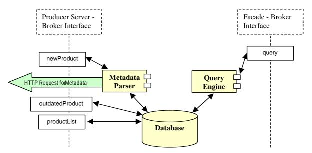
Figure 4.3 The Broker Internal Structure.
