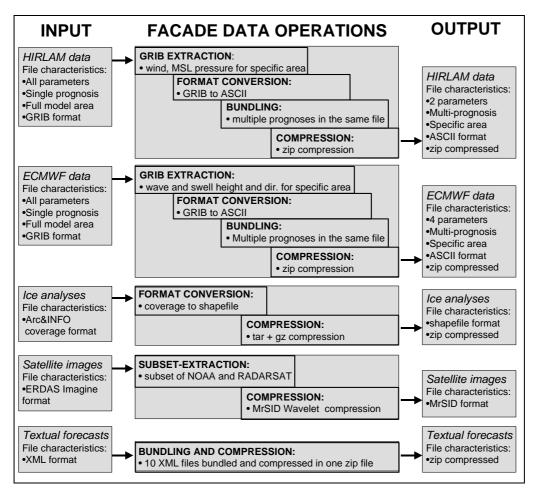
Figure 6.6 A schematic representation of the Facade data operation module.
