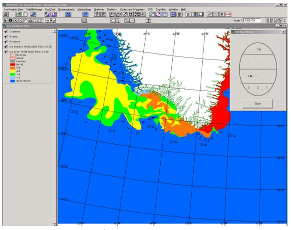
Figure 5.5 An ice analysis from 19<sup>th</sup> of July 2002 represented by a colour code. The Ice Egg Viewer is shown in upper right corner. Clicking ice polygons will reflect the WMO ice egg codes in the Ice Egg Viewer. A graticule has been applied on top of the ice analysis.
