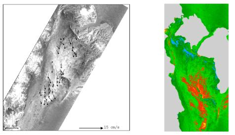
Figure 5.16 Ice motion vectors overlaid on geo-referenced SAR image and ice type classification of the same image. Colour coding of ice classification: blue=open water or thin ice; green=first-year ice; red-yellow=rough first-year ice.
