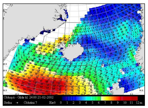
*Figure 5.8* Numerical forecast of ocean waves. Significant wave height in meters is indicated by a colour scale, mean wave direction is shown with an arrow but mean wave period in seconds is given by a number. The forecast is based on the ECMWF wave model.
