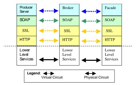
Figure 4.6 The SOAP Based Communication in the Broker Interfaces.
