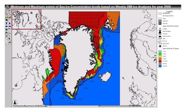
Figure 6.11 Example of the HTML viewer showing sea ice information. The coloured ice chart is a situation in June represented as a weekly chart, overlayed by a hatched layer indicating minimum/maximum limits for ice concentration > 4/10 for year 2000. Note other client features like the toolbar to the left, the legend to right and an overview map in upperleft corner.
