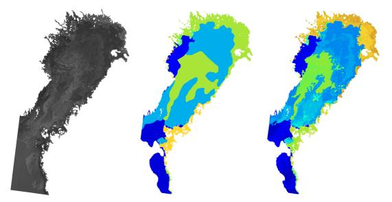
Figure 5.2 A RADARSAT ScanSAR Wide image (© Radarsat), January 25th 2002 [left], and the ice thickness image derived from the digital ice chart of the same day [middle], and an augmented thickness map, based on the simultaneous SAR data [right]. The thickness is coded from blue colour (thin) to red (thick), open sea and land areas are shown in white.
