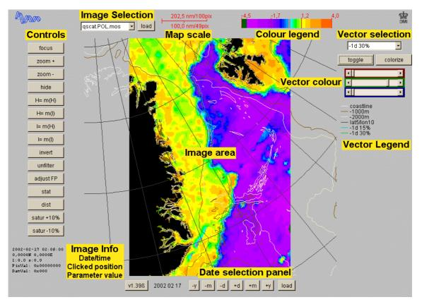
Figure 6.14 The screen layout of the DTU/DCRS JAVA browser for weather, ice and ocean information.
