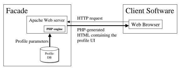
Figure 6.2 The profile editing user interface is implemented using PHP.
