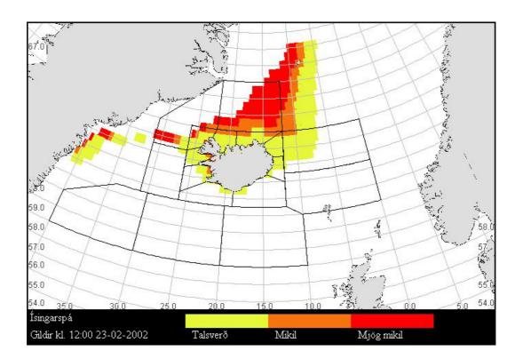
*Figure 5.9* The map shows forecast icing classes calculated by the algorithm of Overland described in the text and *Table 5.2*. The icing classes are Moderate (yellow), Heavy (orange) and Extreme (red).
