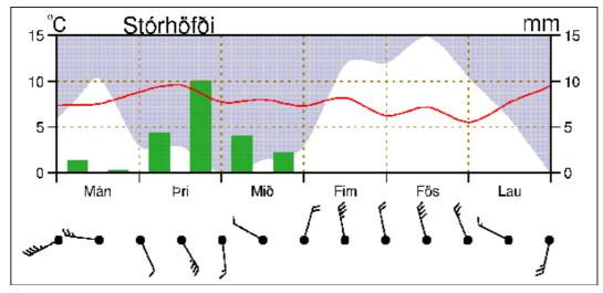
*Figure 5.10* A meteogram showing a six days forecast for the synoptic station Stórhöfði off the south coast of Iceland. Wind speed is shown with flags where one whole barb denotes 5 m/s and a half barb 3 m/s. Air temperature is shown with a red line and accumulated precipitation with green columns. Cloud cover is shown with a bluish background.
