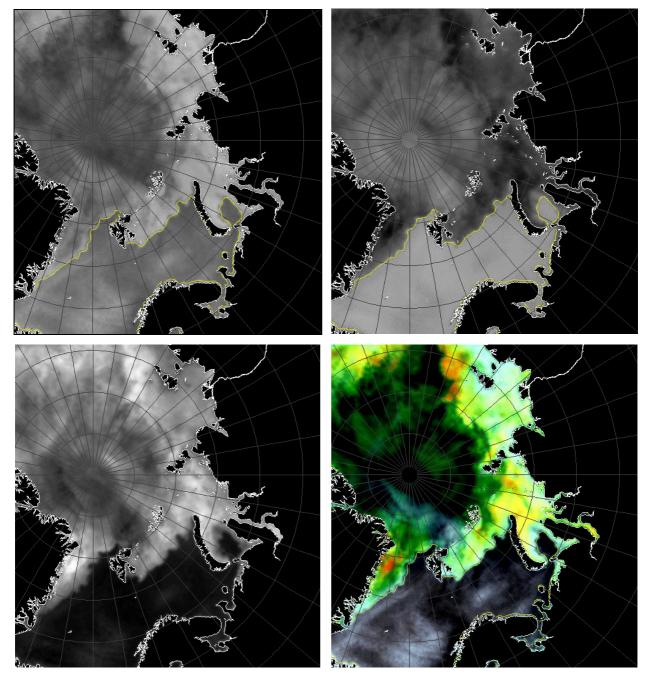
Figure 5.12 AMSU passive microwave products generated in the DTU/DCRS processing chain. These products are generated within a few hours of satellite acquisition, and provide a very useful overview of the large scale ice conditions. Top left is the 89 GHz channel image, upper right is the difference between 150 and 89 GHz, and lower left is the ratio of the same two channels. The lower right image shows an HIS colour combination of the three other images.
