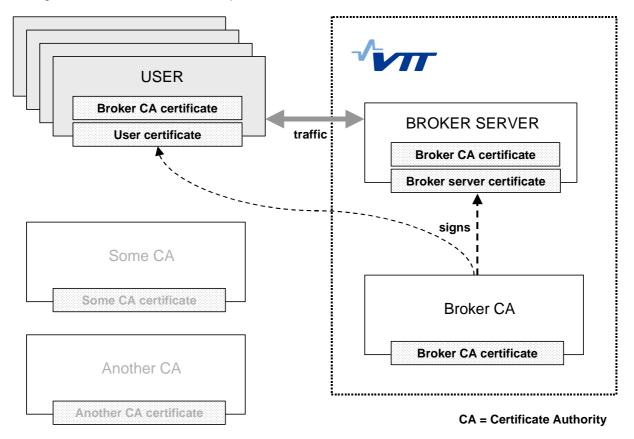
Figure 4.5 Certificates are used in the Extended IWICOS System to make sure that the communicating parties are properly identified.
