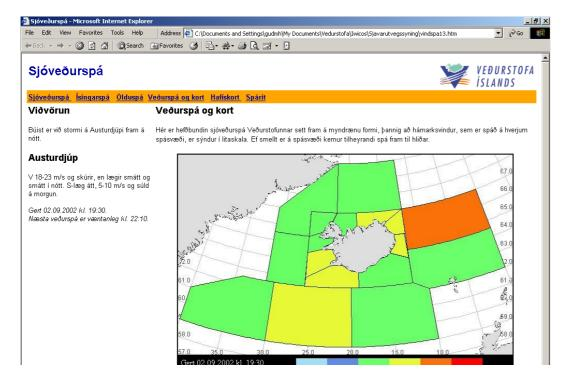
*Figure 6.15* Screen capture from the thin client showing forecast areas coloured according to forecasted wind speed.
