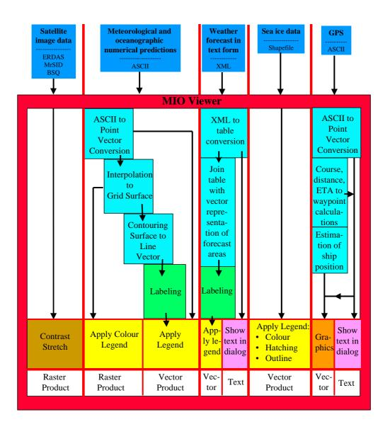
Figure 6.7 MIO Viewer processing chain and display process.
