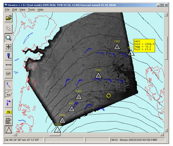
Figure 6.5 Viewlce presenting Radarsat image, buoy observations (triangles), wind and pressure forecast, and ship's location (yellow ring).
