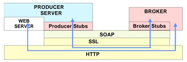
Figure 4.4 Stub Example - The IWICOS Producer Server and Broker Stubs.
