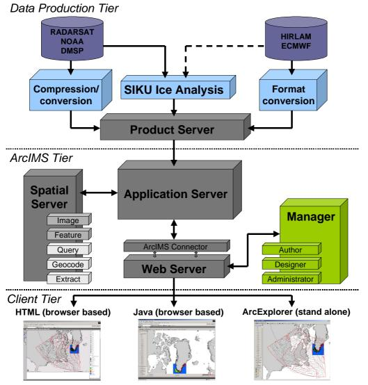
Figure 6.10 Schematic representation of the ArcIMS implementation within IWICOS.
