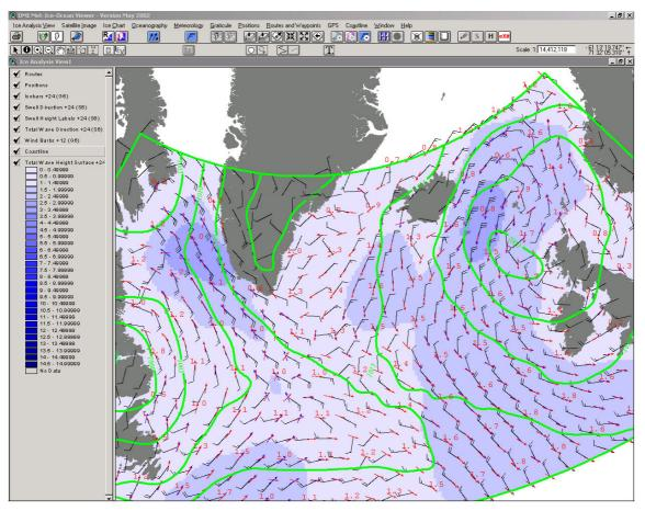
Figure 5.3 An integrated case revealing the strong advantage of having more than one way of representing each parameter. In this case 7 parameters are presented at the same time: Total Wave Height (the coloured surface); Total Wave Direction (blue vectors); Swell Height (red text labels); Swell Direction (red vectors); Wind speed and direction (black wind barbs); MSL Pressure (green isobars).
