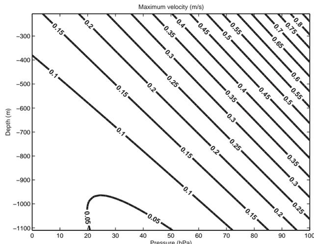
Figure 1: *Maximum velocity as function of depth and pressure depression*
