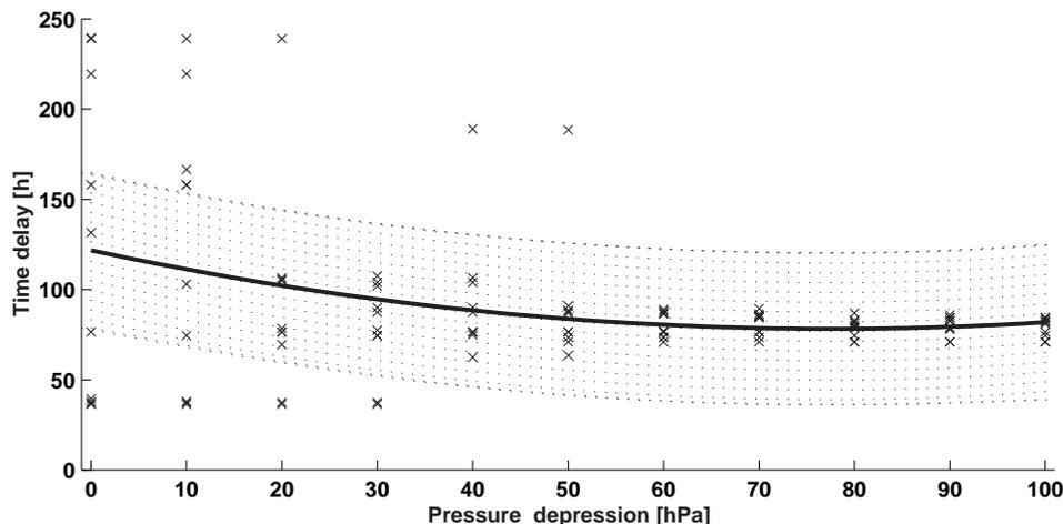
Figure 2: *Regression analysis of time delay of maximum velocity as function of pressure depression. Crosses show data points from Tab. 2 on the preceding page, the line with error-bars show the regression curve written in Eq. (2)*
