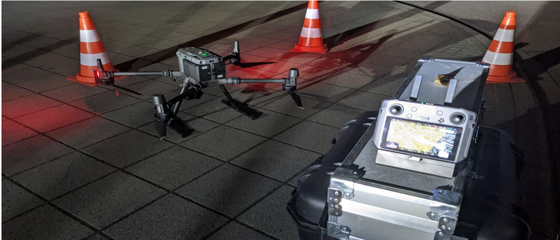
Fig. 4: Experimental setup for UAS flights in Karlsruhe, Germany, including the UAV itself (DJI Matrice 300) and portable control device
