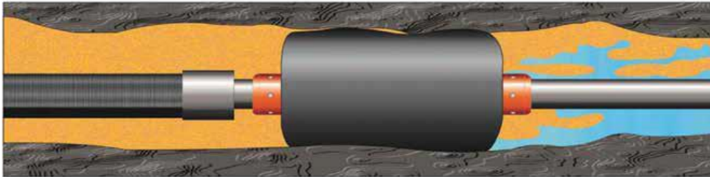
Figure 5: Hybrid packer in the well
