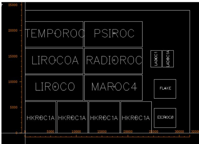
Figure 5: Chip placement in the reticle..
