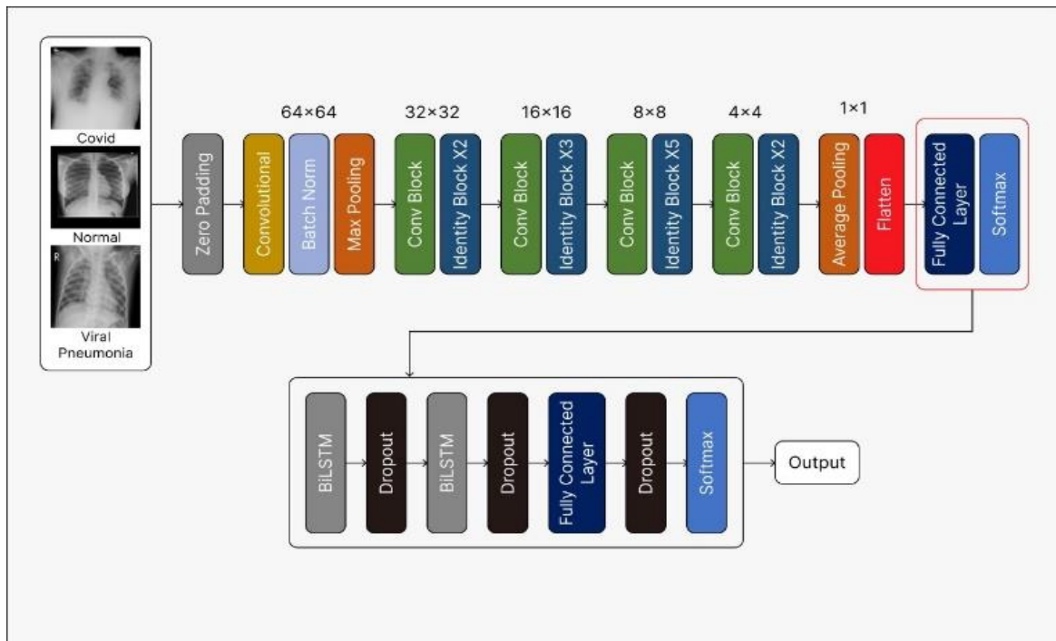
Figure 2. The Resnet50-BiLSTM architecture
