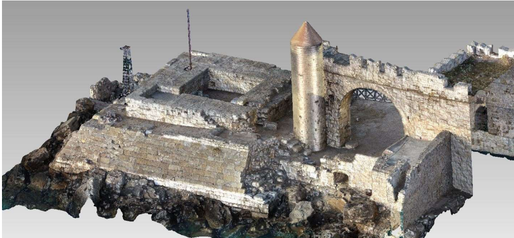
Figure 34: The final, combined dense point cloud for the Naillac Tower in Rhodes.
