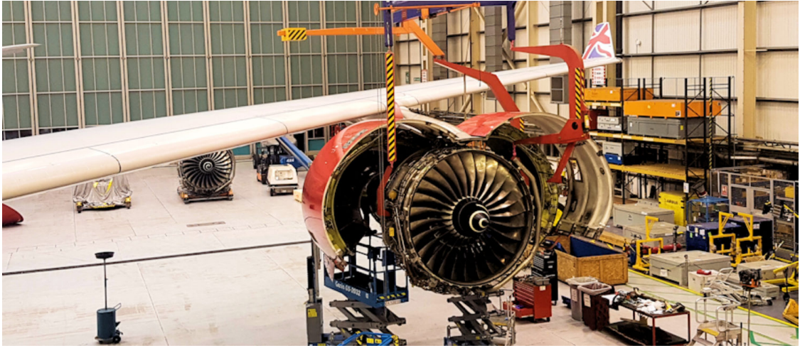
Figure 3.13: Removal of the Rolls Royce Trent 500 engine on an Airbus A340-600 [48].
