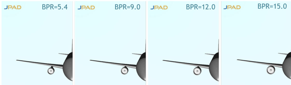
Figure 3.4: Reference engine (to the left) compared with the advanced engines suitable for AGILE regional turbofan aircraft.
