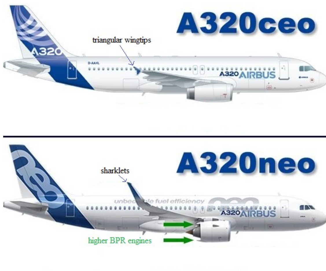
Figure 2.12: A side-by-side comparison of the Airbus A320ceo and A320neo [34].
