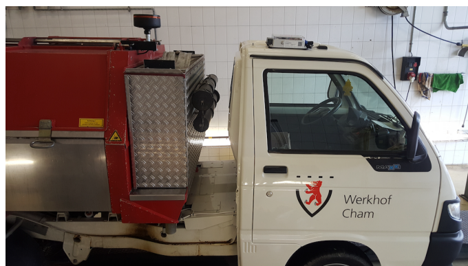
Figure 4. Sensor-box mounted on a utility vehicle from the municipality of Cham.
