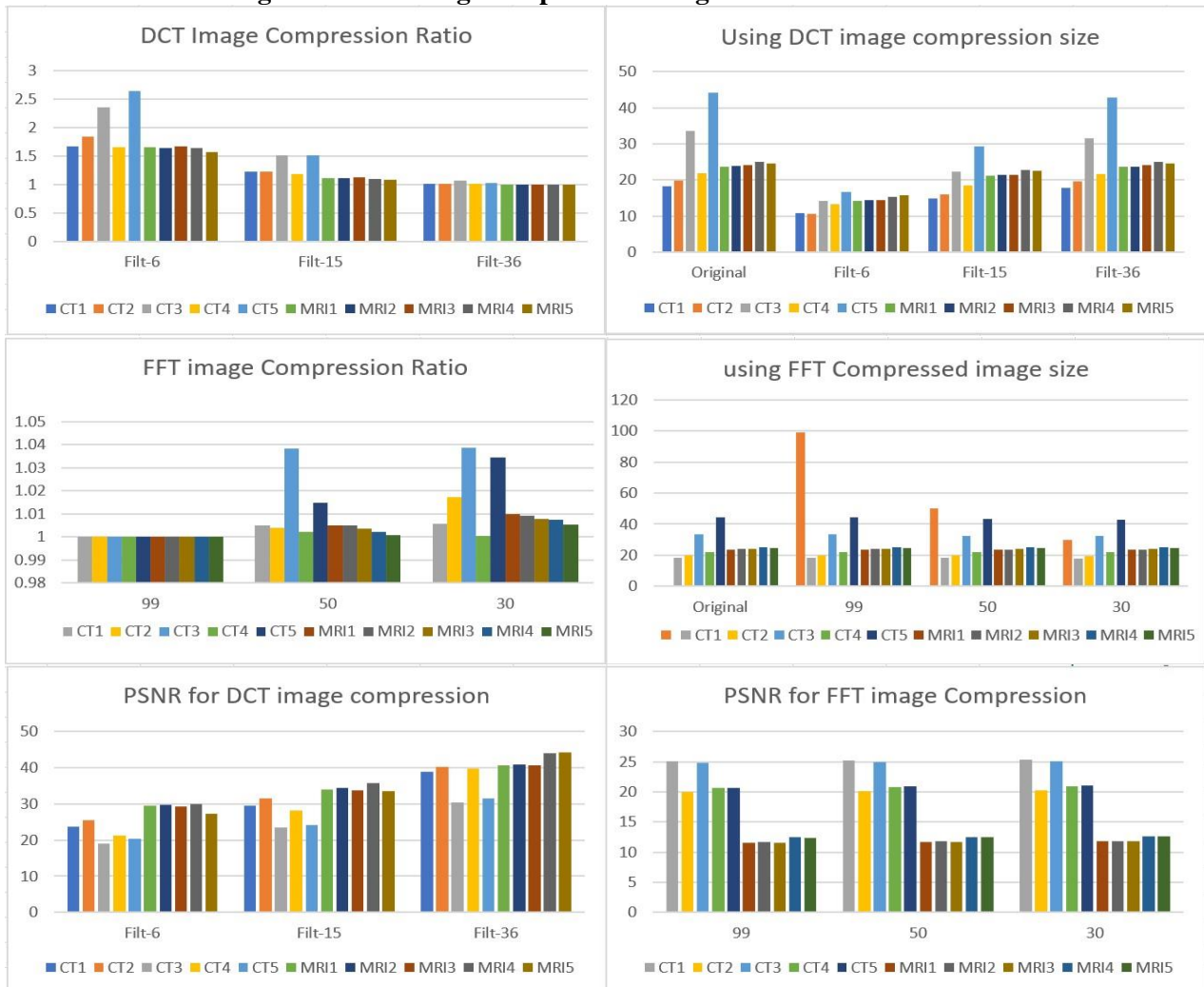
Figure 5. Graph shows CR, PSNR and compressed size of the image were evaluation values take 512x512 size of 5 CT images and 5 MRI images with DCT and FFT.
