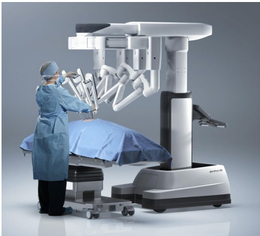
Figure 2. The da Vinci Surgical System patient-side cart (Figure courtesy of Intuitive Surgical, Inc. - The copyrights are protected by Intuitive)
