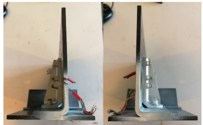
Figure 22. Lateral edges of the mouse hole specimen 1 after failure.
