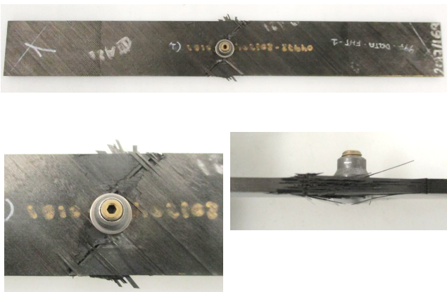
Figure 9. Example of FHT failure mode.
