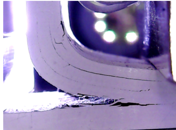
Figure 17. Failure mode of the first unfolding specimen. Similar failure was found in the specimen #2.
