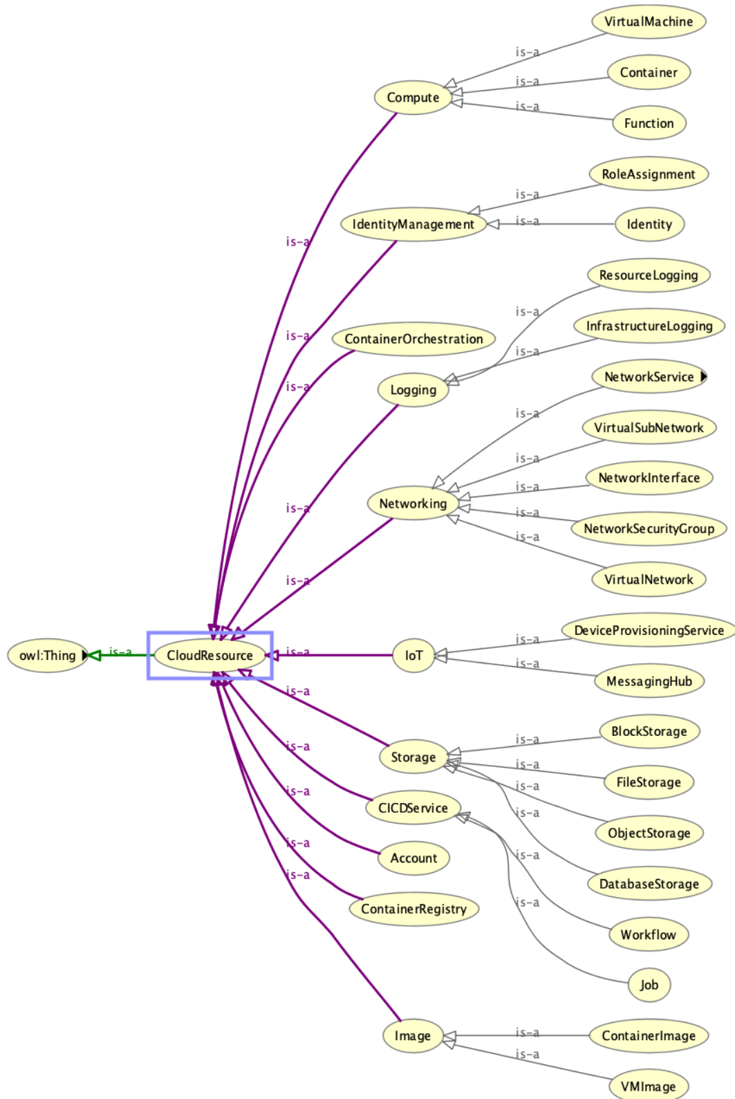
Figure 17. The cloud resource taxonomy which classifies cloud resources according to their functional purpose, like compute, storage, and networking
