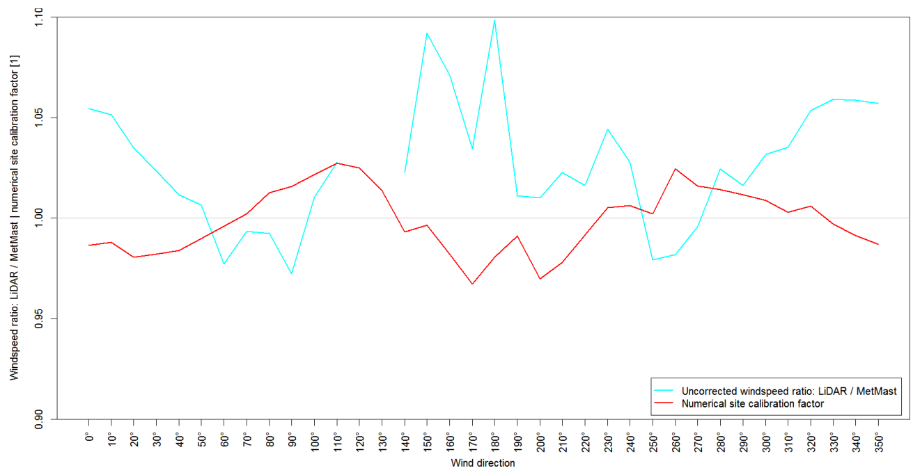
Figure 21: Results for the numerical site calibration for Site C for different wind directions (red line). For comparison, the bin-averaged mean deviations between the LiDAR and met mast measurement have been included as light blue line. This is the same data as shown as light blue line in Figure 9.
