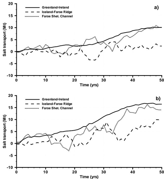
Figure 19: Time series showing the difference compared to CTRL in the annual mean net northward salt transport (Mt) for (a) PX2 and (b) PX5 through the GI section (solid), the IFR (dashed) and the FSC (dotted). Negative values indicate reduced transport.
