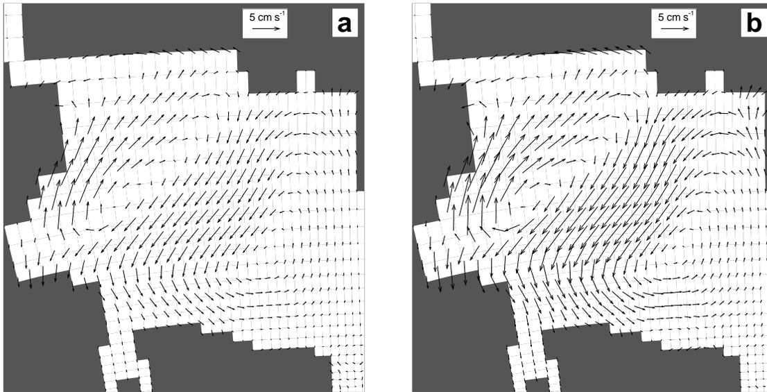
Figure 14: Difference compared to CTRL in the annual mean sea ice velocity ( $\text{cm s}^{-1}$ ) in year 50 for (a) PX2 and (b) PX5.
