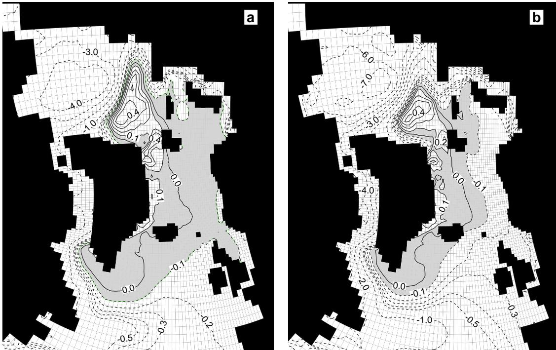
Figure 10: Difference in annual mean sea surface salinity compared to CTRL in year 50. (a) PX2, and (b) PX5. Dotted lines represent negative anomalies. CI is 1 psu. In addition the contour lines from -0.5 to 0.5 psu are shown in CI of 0.1 psu.
