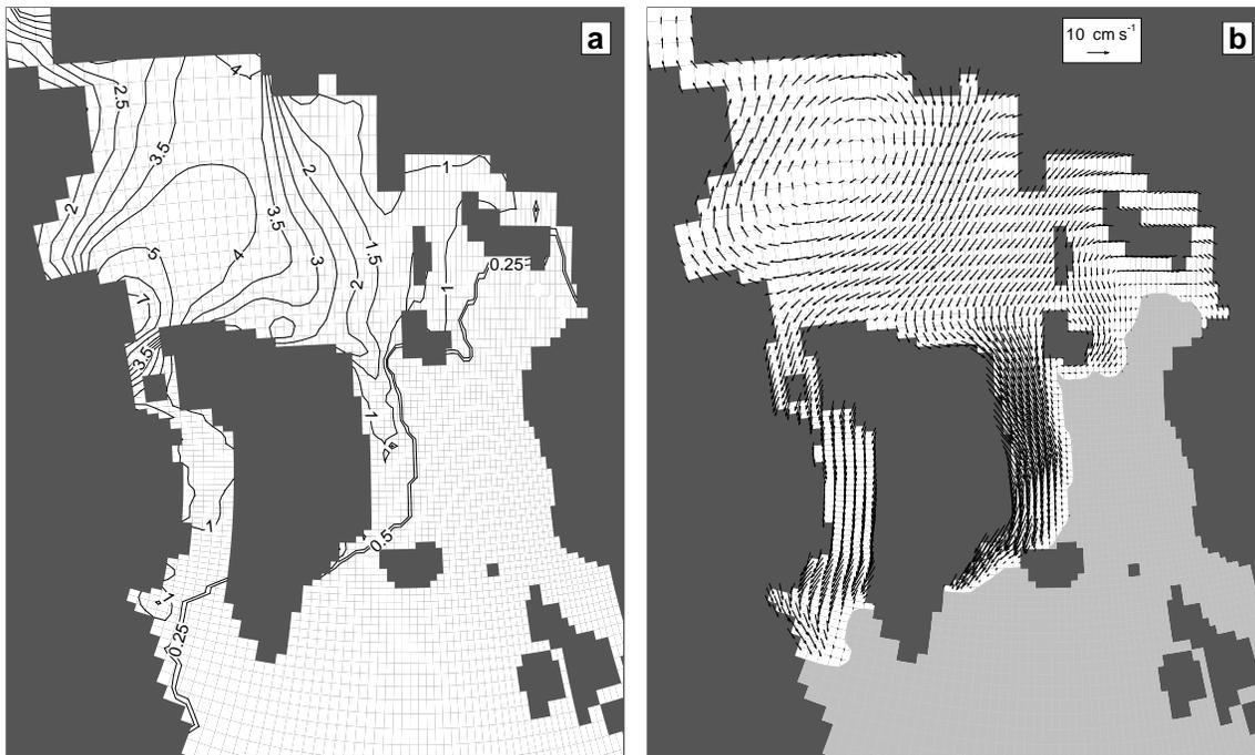
Figure 7: (a) Sea ice thickness (m; left panel) in March at the start of CTRL, and (b) annual mean sea ice velocity ( $\text{cm s}^{-1}$ ) in the first year of CTRL. In panel (a), CI is 0.5 m. In addition the 0.25 m contour level is shown.
