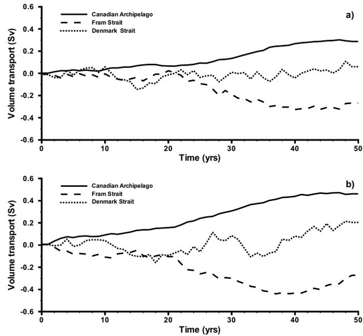
Figure 16: Time series showing the difference compared to CTRL in the annual mean net southward volume transport (Sv) for (a) PX2 and (b) PX5 through the CA (solid line), Fram Strait (dashed) and Denmark Strait (dotted). Negative values indicate reduced transport.
