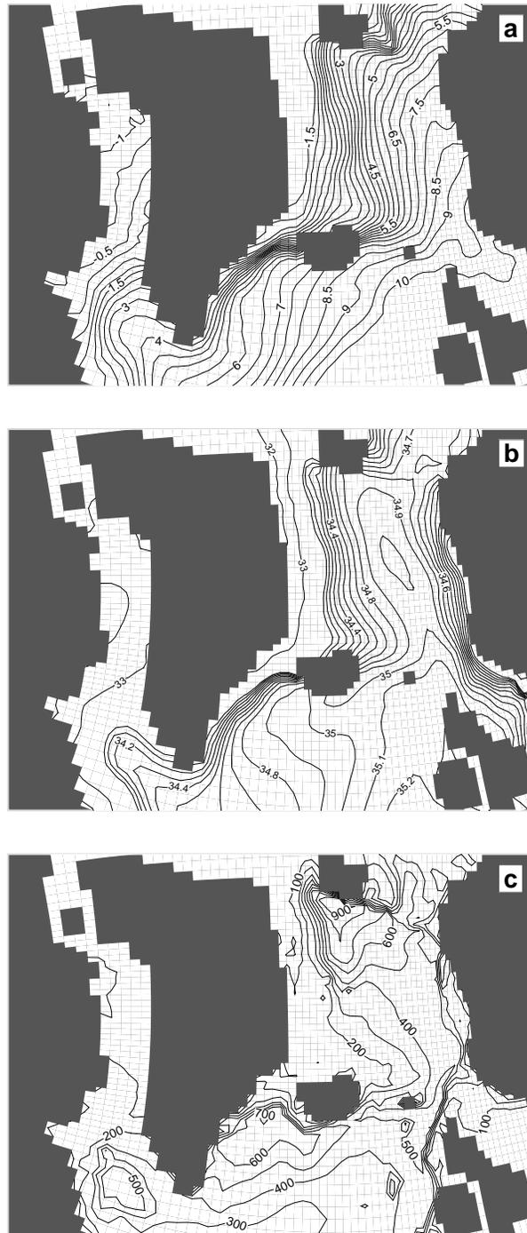
Figure 9: Mixed layer properties for the Nordic Seas and the northern North Atlantic at the start of CTRL. (a) Annual mean sea surface temperature ( $^{\circ}\text{C}$ ), (b) annual mean sea surface salinity (psu) and (c) winter mixed layer thickness (m). CIs are (a)  $0.5^{\circ}\text{C}$ , (b)  $0.1$  psu for contour values  $\geq 34$ , and (c)  $100$  m. In (b) the  $32$  and  $33$  psu contour levels are also shown.
