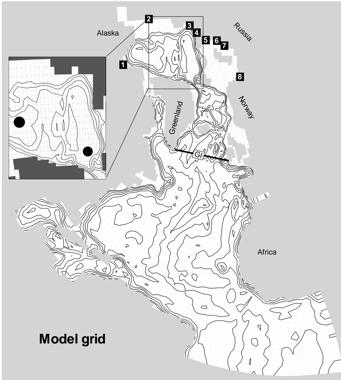
Figure 1: The model grid used in this study. The numbers 1–8 represent the major river discharge locations in the Arctic Ocean (MacKenzie, Kolyma, Kotuy, Lena, Ob, Yenisei, Pyasina and Northern Dvina, respectively). Also shown are two locations in the Arctic Ocean, one in the Eurasian Basin and a second one in the Canadian Basin. Finally, the Greenland-Ireland transect used in the text is shown.
