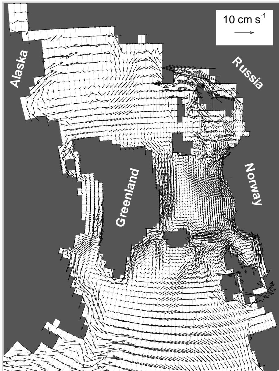
Figure 5: Simulated annual mean sea surface velocity field ( $\text{cm s}^{-1}$ ) at the start of CTRL.
