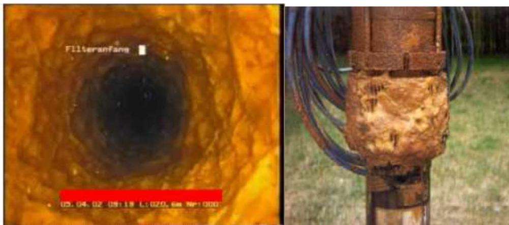
**Figure 1:** left: clogged well, ochre deposits inside the screen; right: clogged pump, ochre deposits at the pump intake, both ©BWB
