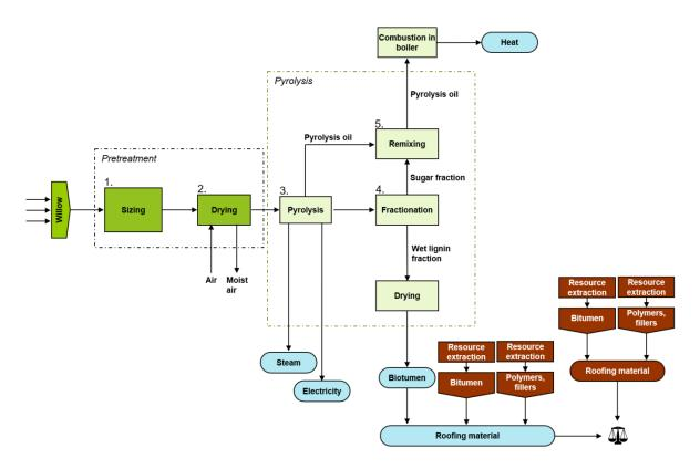
Figure 51: Detailed life cycle comparison for VC 4: biotumen from willow via pyrolysis versus bitumen from fossil resources. A more detailed scheme for the pyrolysis section can be found in Figure 48.
