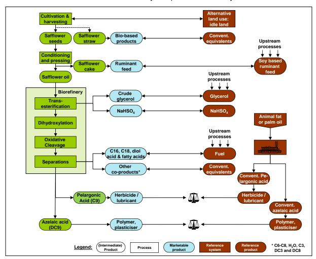
Figure 42: Simplified life cycle comparison for VC 5: organic acids from safflower via oxidative cleavage versus organic acids from fossil resources.
