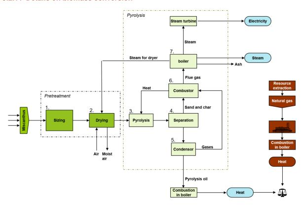
Figure 48: Detailed life cycle comparison for VC 1: industrial heat from Miscanthus via pyrolysis versus industrial heat from fossil energy carriers.
