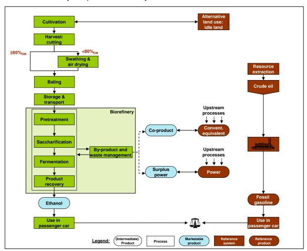
Figure 40: Simplified life cycle comparison for VC 3: ethanol from switchgrass via hydrolysis and fermentation versus fossil gasoline.
