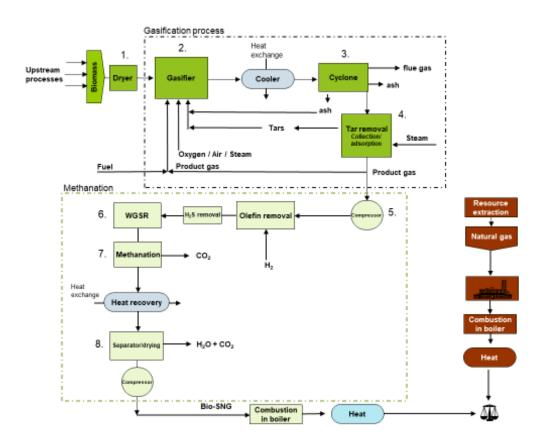
Figure 49: Detailed life cycle comparison for VC 2: Synthetic natural gas from poplar via gasification versus natural gas.
