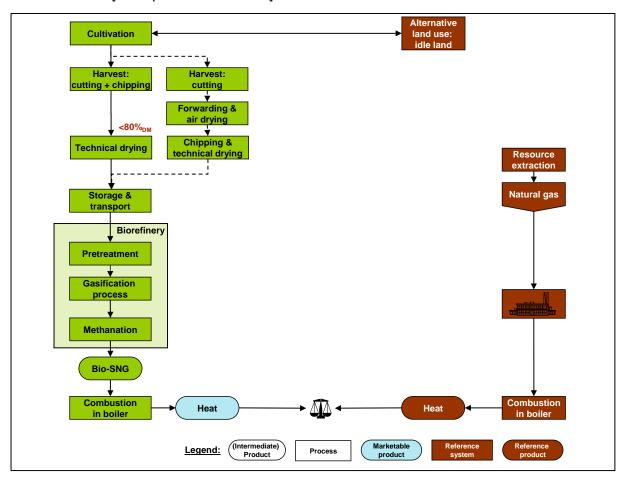
Figure 39: Simplified life cycle comparison for VC 2: synthetic natural gas from poplar via gasification versus natural gas.
