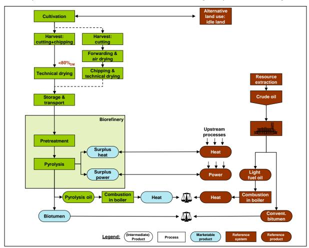
Figure 41: Simplified life cycle comparison for VC 4: biotumen from willow via pyrolysis versus bitumen from fossil resources.
