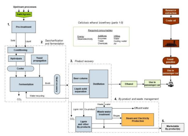
Figure 50: Detailed life cycle comparison for VC 3: ethanol from switchgrass via hydrolysis & fermentation versus fossil gasoline.
