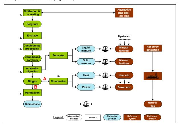
Figure 46: Life cycle comparison for VC 9: biogas/biomethane from sorghum versus natural gas.
