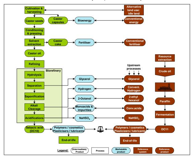
Figure 44: Simplified life cycle comparison for VC 7: products derived from sebacic acid from castor oil versus the same products from paraffins derived through fermentation of petroleum<sup>7</sup>.
