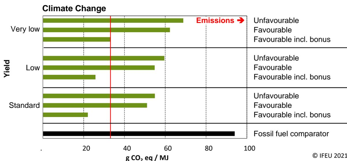
Figure 36: GHG emissions according to RED II for bioethanol from switchgrass (via hydrolysis and fermentation) compared to the fossil fuel comparator (black bar). The red line illustrates 65% GHG emissions savings threshold, that biofuels must not exceed.
