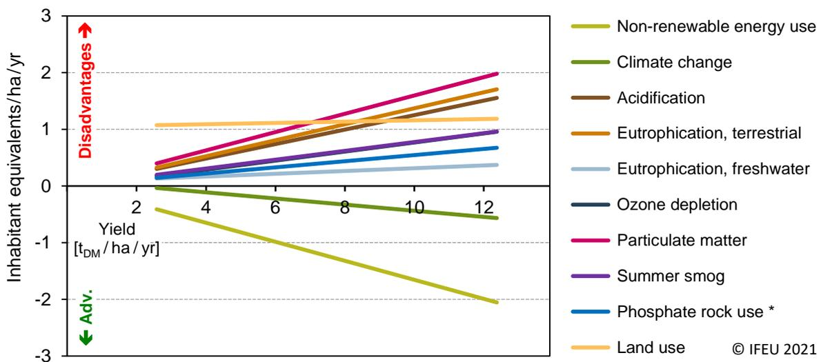
Figure 14: LCA results for synthetic natural gas from poplar (via gasification) versus natural gas. \* results for phosphate rock use: multiply by 10.
