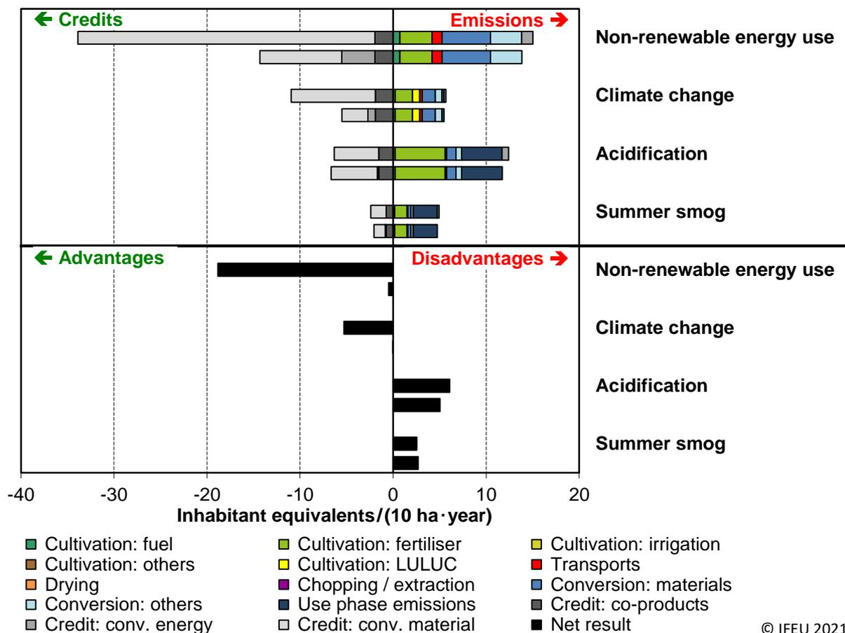
Figure 29: LCA results for hemp-based insulation versus conventional insulation from mineral wool (upper bars) and from EPS (lower bars), respectively, at a yield level of 8.0 t<sub>DM</sub>/ha/yr.
