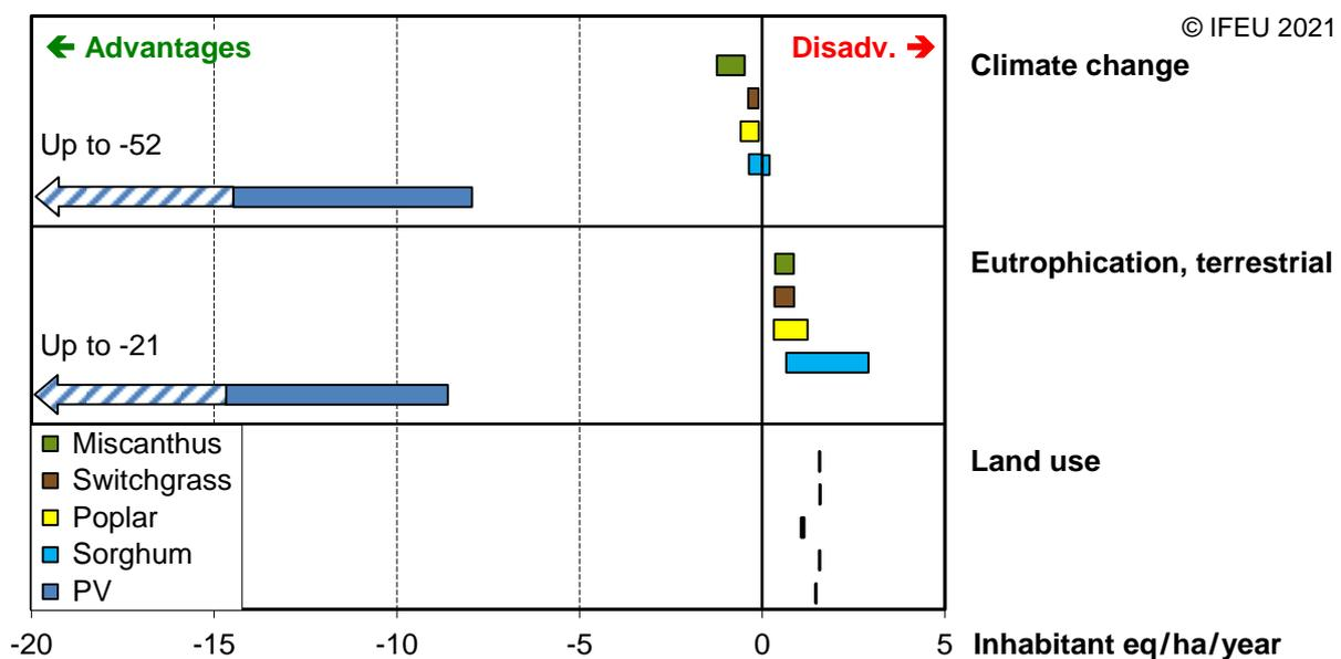
Figure 35: LCA results for renewable electricity from a PV system on marginal land compared to four exemplary bioenergy products: heat from Miscanthus, ethanol from switchgrass, synthetic natural gas from poplar and biogas/biomethane from sorghum (see results in section 4.2). The results for PV cover different intensities of solar irradiation from the MED to the CON zone.
