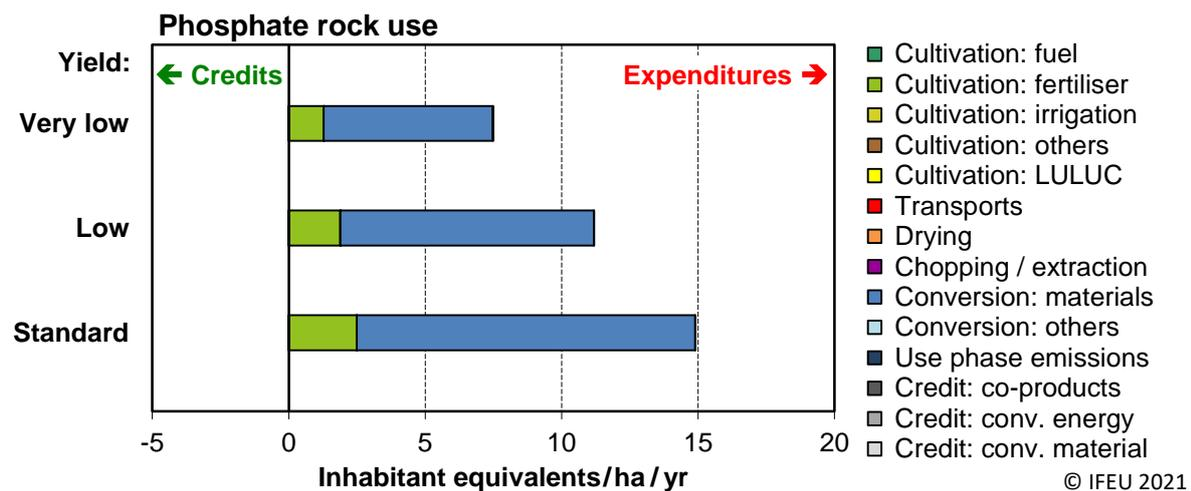
Figure 18: LCA results for ethanol from switchgrass (via hydrolysis and fermentation) versus fossil gasoline for the impact category phosphate rock use. Results are given for three yield levels in the Mediterranean zone.
