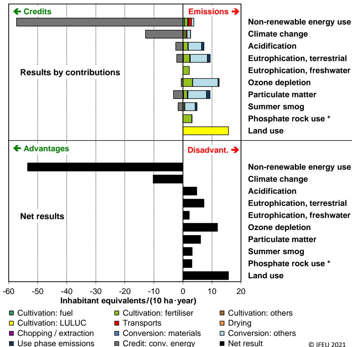
Figure 7: Normalised LCA results (given in inhabitant equivalents) for all impact categories for industrial heat from Miscanthus compared to industrial heat from natural gas at a yield of 12.5 t<sub>DM</sub>/ha/yr. Upper panel: results by contributions of individual life cycle steps. Lower panel: net results. \* results for phosphate rock use: multiply by 10.
