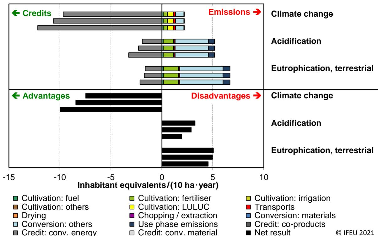
Figure 13: Impact of the energy carrier used for conventional heat production on the LCA results for industrial heat from Miscanthus versus industrial heat from natural gas (upper bars), from light fuel oil (middle bars) and from coal (lower bars) for selected impact categories.
