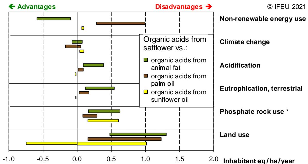
Figure 23: LCA results for organic acids from safflower versus conventional organic acids from animal fat, palm oil and sunflower oil for yield levels ranging from “Very low” to “Standard”. \* results for phosphate rock use: multiply by 10.
