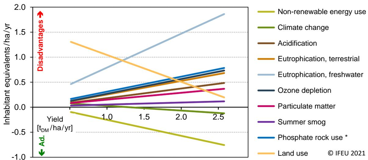
Figure 21: LCA results for organic acids from safflower (via oxidative cleavage) versus conventional organic acids from animal fat. \* results for phosphate rock use: multiply by 10.
