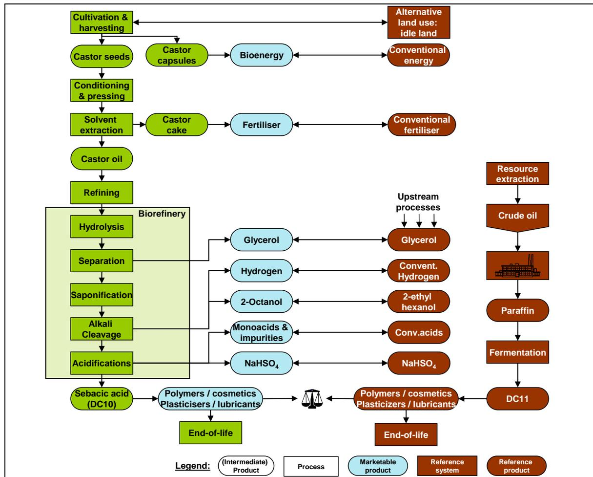
Figure 44: Simplified life cycle comparison for VC 7: products derived from sebamic acid from castor oil versus the same products from paraffins derived through fermentation of petroleum<sup>7</sup>.
