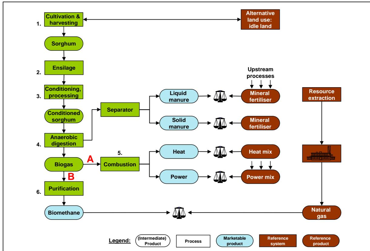
Figure 46: Life cycle comparison for VC 9: biogas/biomethane from sorghum versus natural gas.
