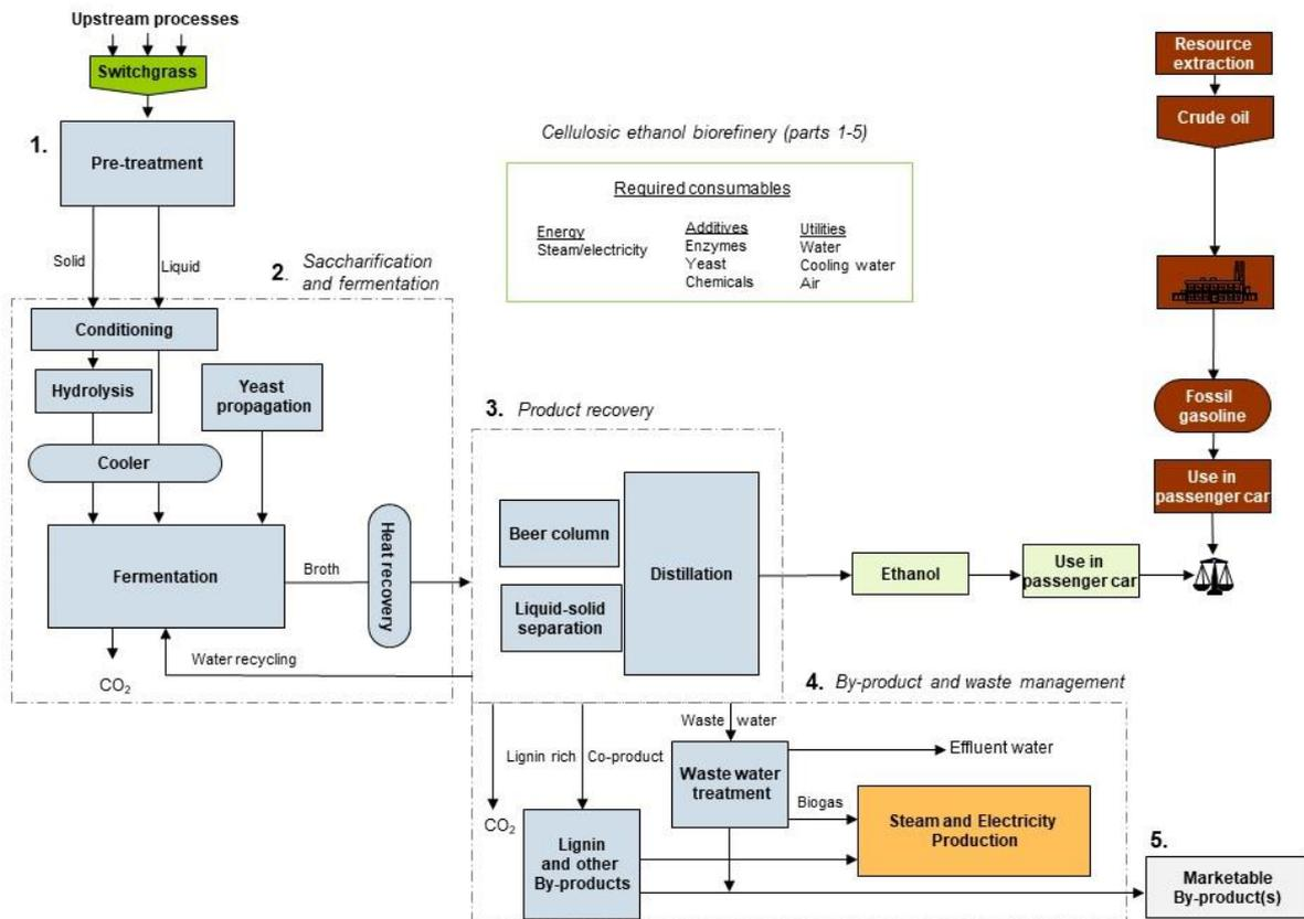
Figure 50: Detailed life cycle comparison for VC 3: ethanol from switchgrass via hydrolysis & fermentation versus fossil gasoline.
