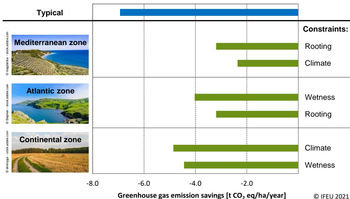
Figure 20: GHG emission savings for biotumen from willow (via pyrolysis) versus conventional bitumen for two biophysical constraints each in the three agro-ecological zones.
