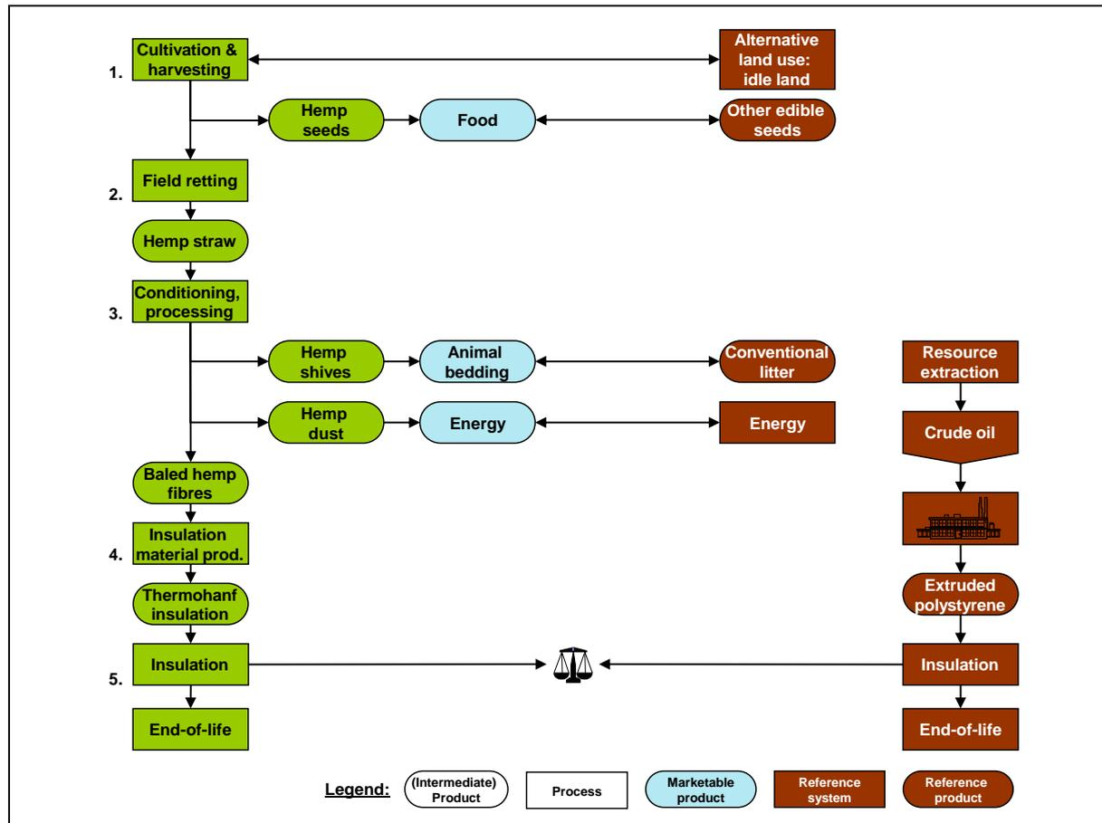
Figure 45: Life cycle comparison for VC 8: insulation material from industrial hemp versus insulation material from fossil resources (e.g. extruded polystyrene).
