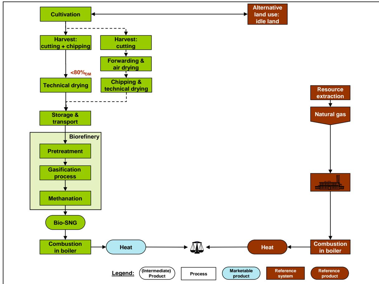
Figure 39: Simplified life cycle comparison for VC 2: synthetic natural gas from poplar via gasification versus natural gas.
