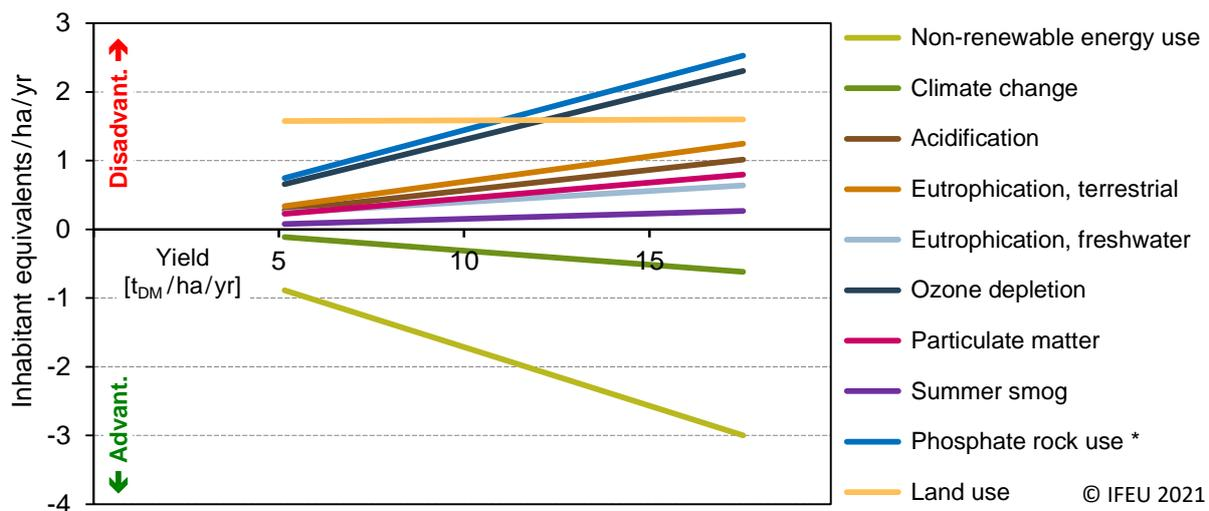
Figure 16: LCA results for ethanol from switchgrass (via hydrolysis and fermentation) versus fossil gasoline. \* results for phosphate rock use: multiply by 10.
