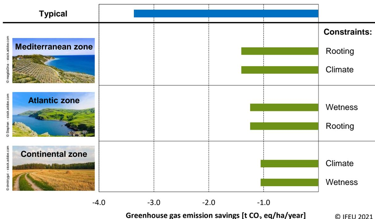
Figure 17: GHG emission savings for ethanol from switchgrass (via hydrolysis and fermentation) versus fossil gasoline for two biophysical constraints each in the three agro-ecological zones.
