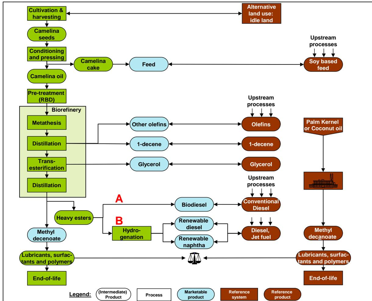
Figure 43: Simplified life cycle comparison for VC 6: methyl decenoate from camelina via metathesis versus methyl decanoate from biogenic resources<sup>6</sup>.
