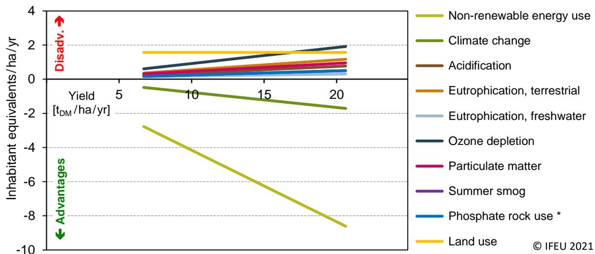
Figure 11: LCA results for industrial heat from Miscanthus (via pyrolysis) versus industrial heat from natural gas. \* results for phosphate rock use: multiply by 10.
