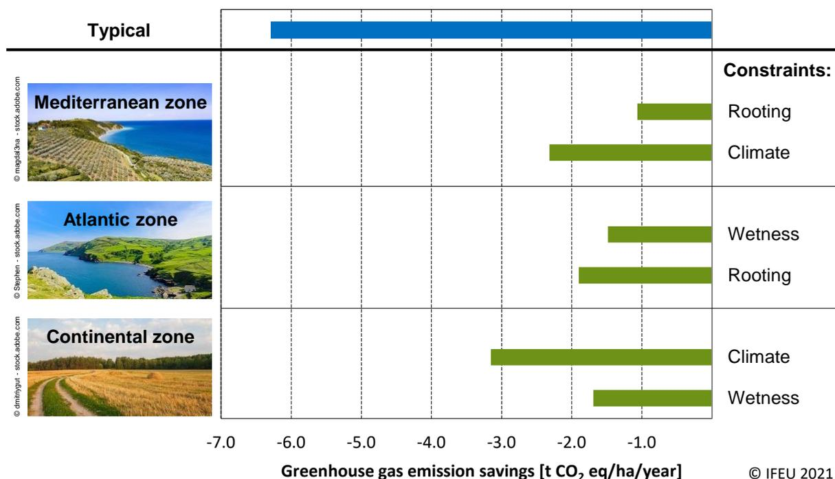
Figure 31: GHG emission savings for heat and power from sorghum biogas versus heat and power mix from fossil energy carriers for two biophysical constraints each in the three AEZ.
