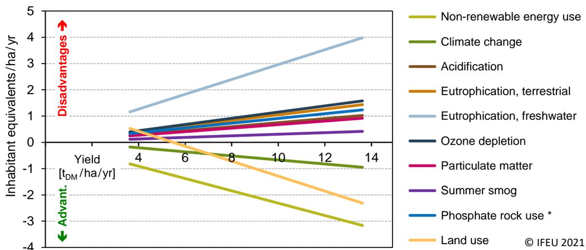
Figure 27: LCA results for insulation material from hemp versus conventional EPS. \* results for phosphate rock use: multiply by 10.
