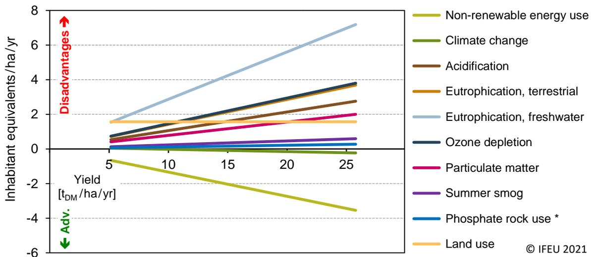
Figure 32: LCA results for biomethane from sorghum versus natural gas. \* results for phosphate rock use: multiply by 10.
