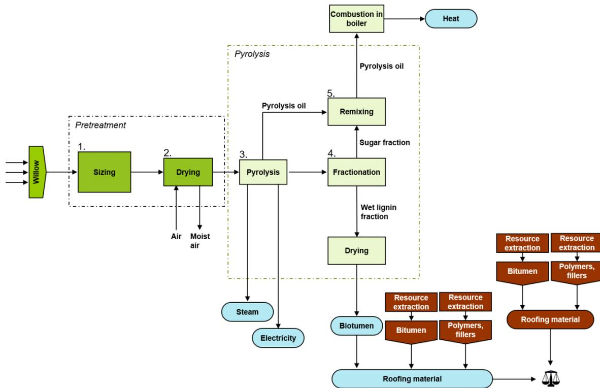
Figure 51: Detailed life cycle comparison for VC 4: biotumen from willow via pyrolysis versus biotumen from fossil resources. A more detailed scheme for the pyrolysis section can be found in Figure 48.
