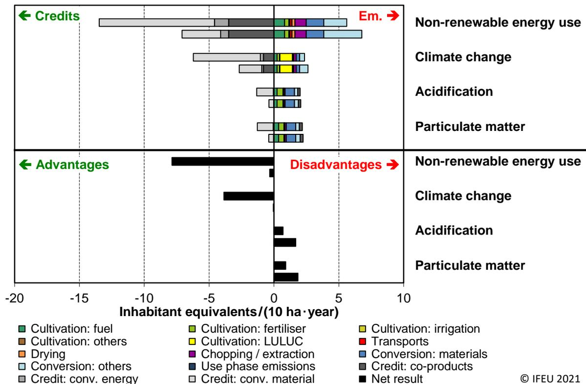
Figure 26: LCA results for sebacic acid from castor (via alkaline cleavage) versus sebacic acid from paraffin at a yield level of 1.3 t<sub>DM</sub>/ha/yr. The best case and the worst case scenario, respectively upper and lower bars, are presented for each category.
