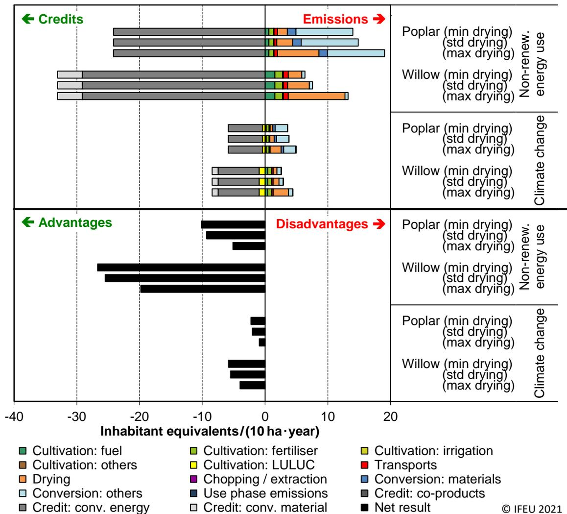
Figure 37: Normalised LCA results (inhabitant equivalents) of non-renewable energy use and climate change for natural gas from poplar (via gasification) versus natural gas and for biotumen from willow (via pyrolysis) versus conventional bitumen for yields of 5.5  $t_{DM}/ha/yr$  (poplar) and 7.5  $t_{DM}/ha/yr$  (willow), respectively.
