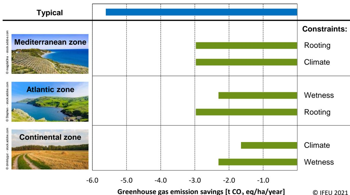
Figure 28: GHG emission savings for insulation material from hemp versus conventional EPS for two biophysical constraints each in the three agro-ecological zones.
