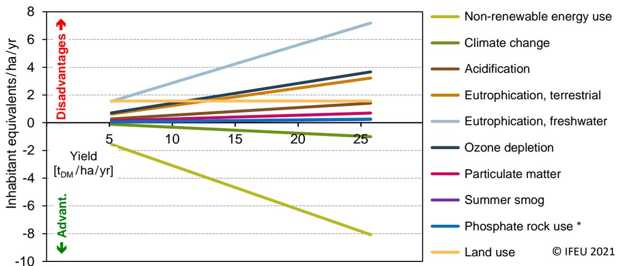
Figure 30: LCA results for heat and power from sorghum biogas versus heat and power mix from fossil energy carriers. \* results for phosphate rock use: multiply by 10.
