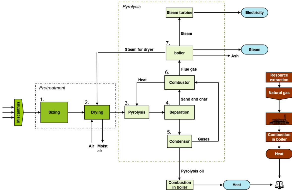
Figure 48: Detailed life cycle comparison for VC 1: industrial heat from Miscanthus via pyrolysis versus industrial heat from fossil energy carriers.
