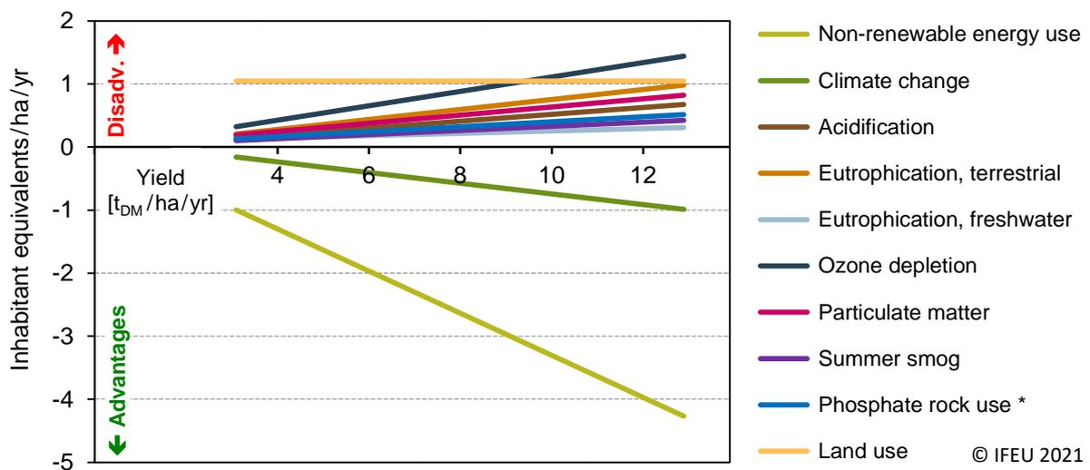
Figure 19: LCA results for biotumen from willow (via pyrolysis) versus conventional bitumen. \* results for phosphate rock use: multiply by 10.
