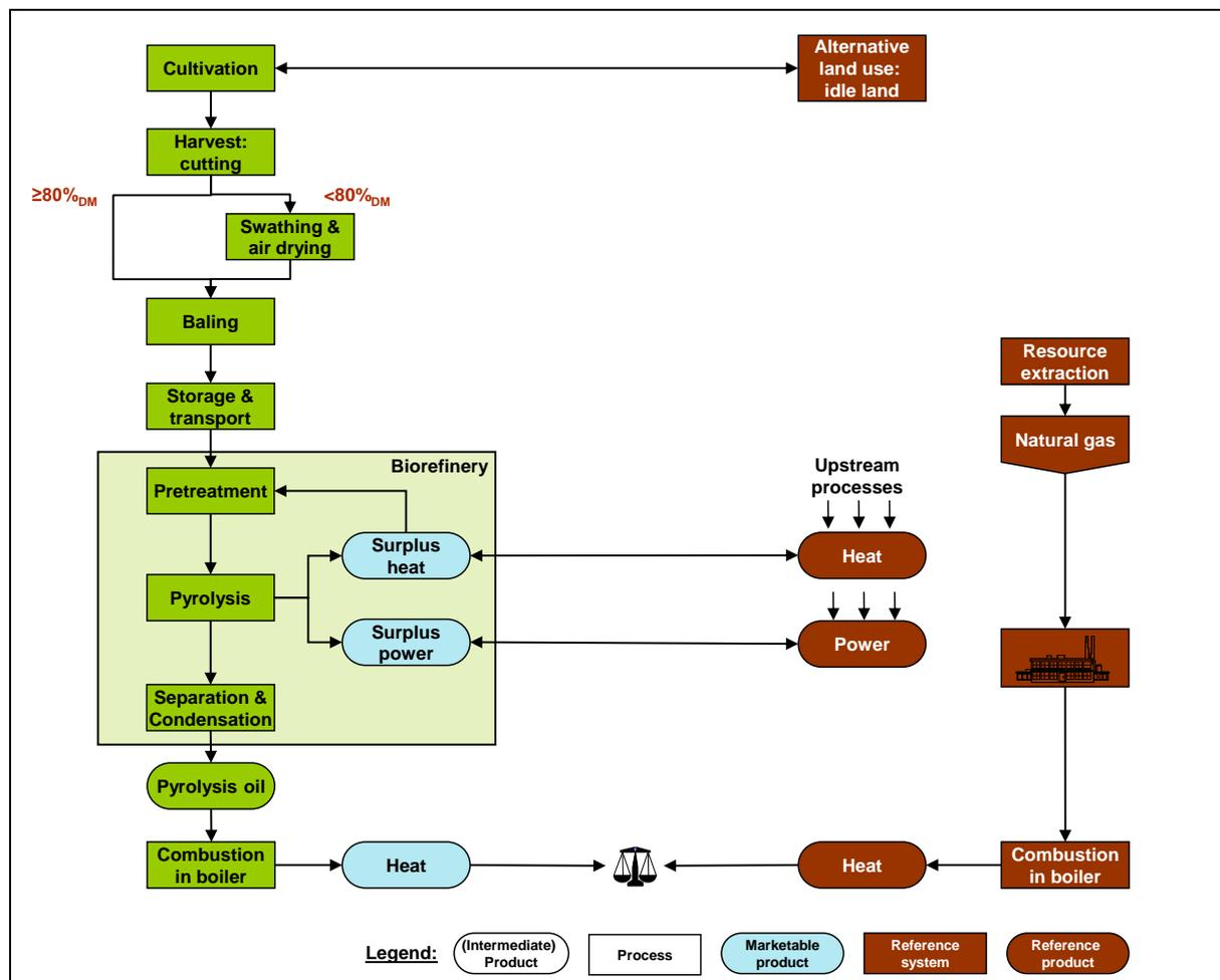
Figure 38: Simplified life cycle comparison for VC 1: industrial heat from Miscanthus via pyrolysis versus industrial heat from fossil energy carriers.
