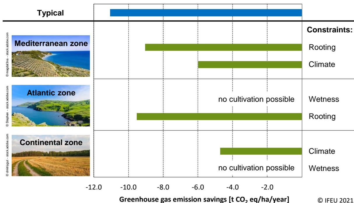
Figure 12: GHG emission savings for industrial heat from Miscanthus (via pyrolysis) versus industrial heat from natural gas for two biophysical constraints each in the three agro-ecological zones.
