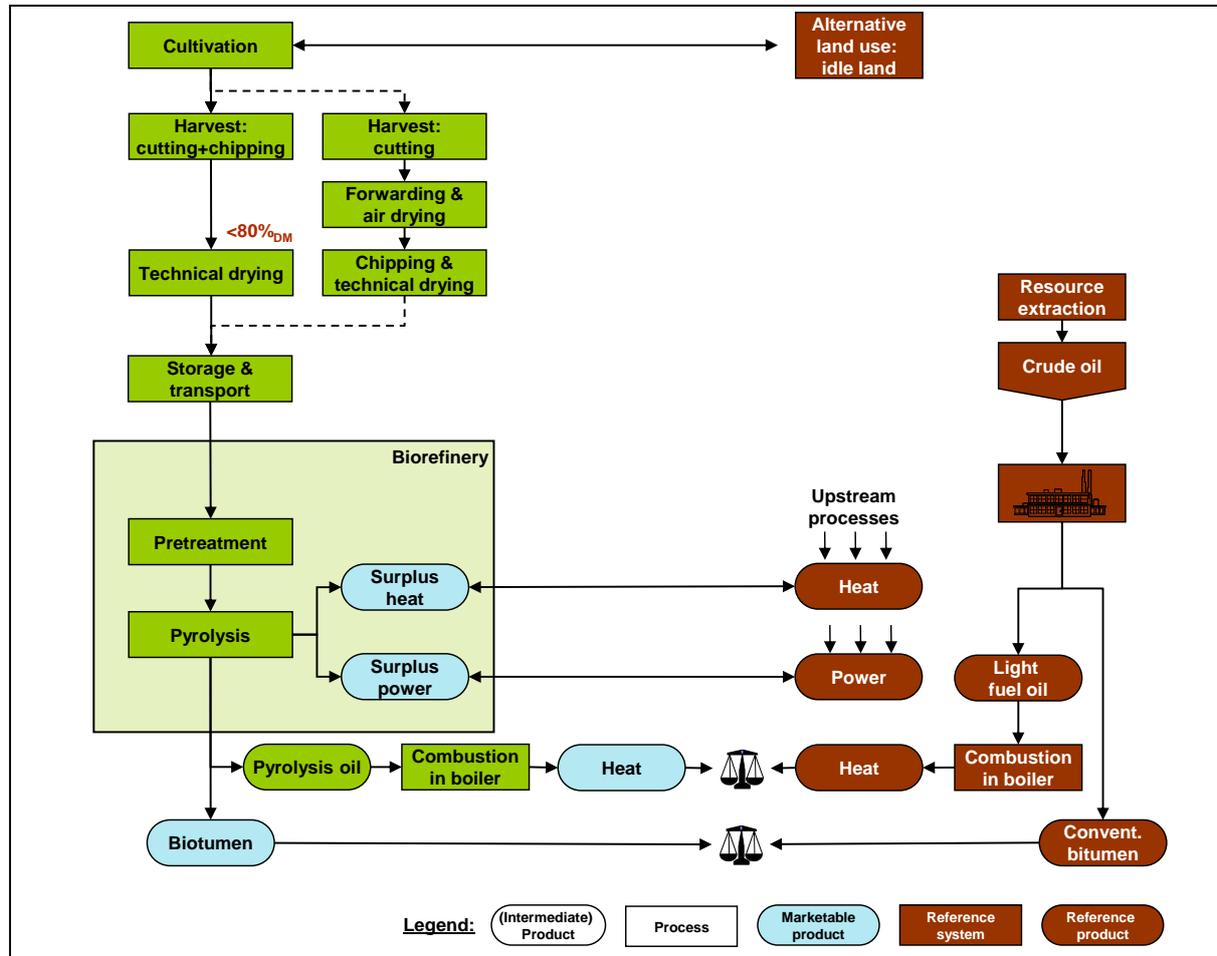
Figure 41: Simplified life cycle comparison for VC 4: biotumen from willow via pyrolysis versus bitumen from fossil resources.
