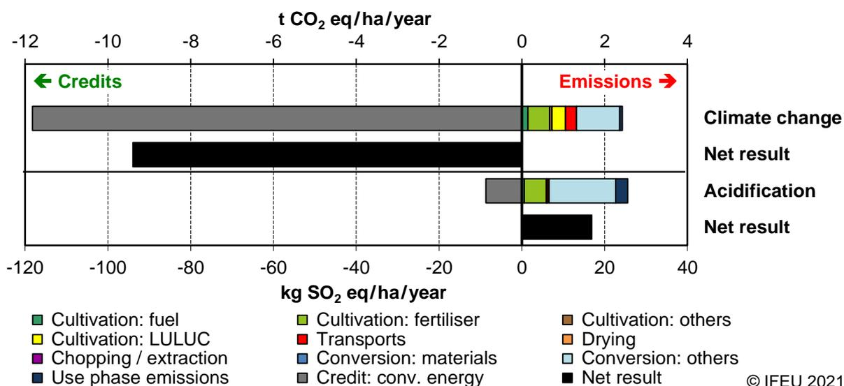
Figure 6: LCA results for industrial heat from Miscanthus compared to industrial heat from natural gas for the impact categories climate change and acidification at a yield of 12.5 t<sub>DM</sub>/ha/yr.
