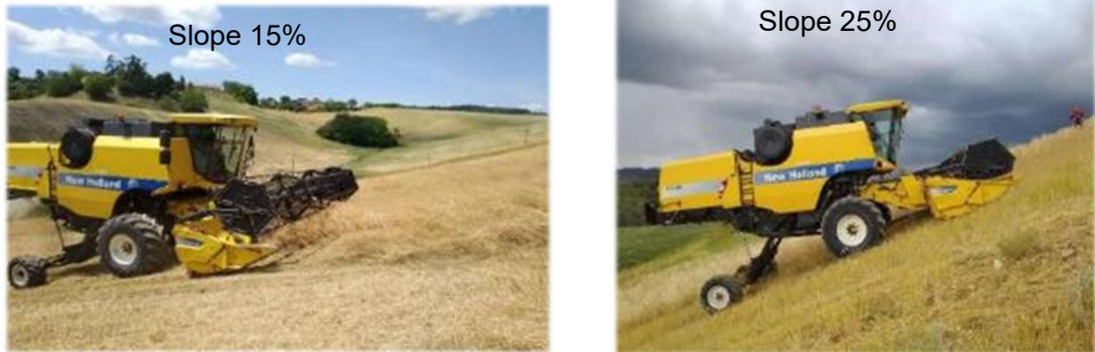
Figure 1 UNIBO. Experimental fields with different slopes during camelina harvest in 2020.
