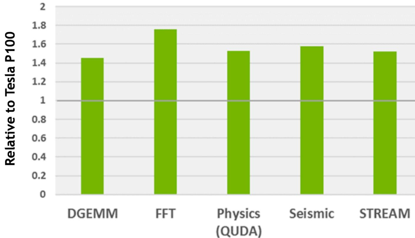
System Config Info: 2X Xeon E5-2690 v4, 2.6GHz, w/ 1X Tesla P100 or V100. V100 measured on pre-production hardware.
