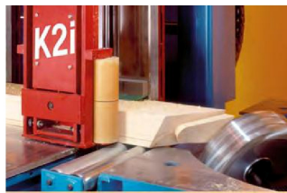
Figure 1 Hundegger K2i working on a Dovetail (Hans Hundegger AG, p. 21); These robots represent affordable and ready-to-use solutions for a carpenter workshop. Even though they optimize issues like precision, speed and complexity of the manufacturing process, they definitely change the workflow and skill of a carpenter.
