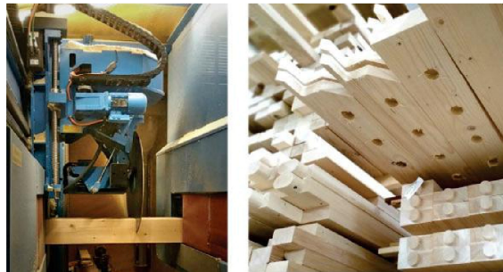
Figure 1. A joinery robot (left) is able to produce round wooden studs (right) or dovetail joints quickly and accurately.
