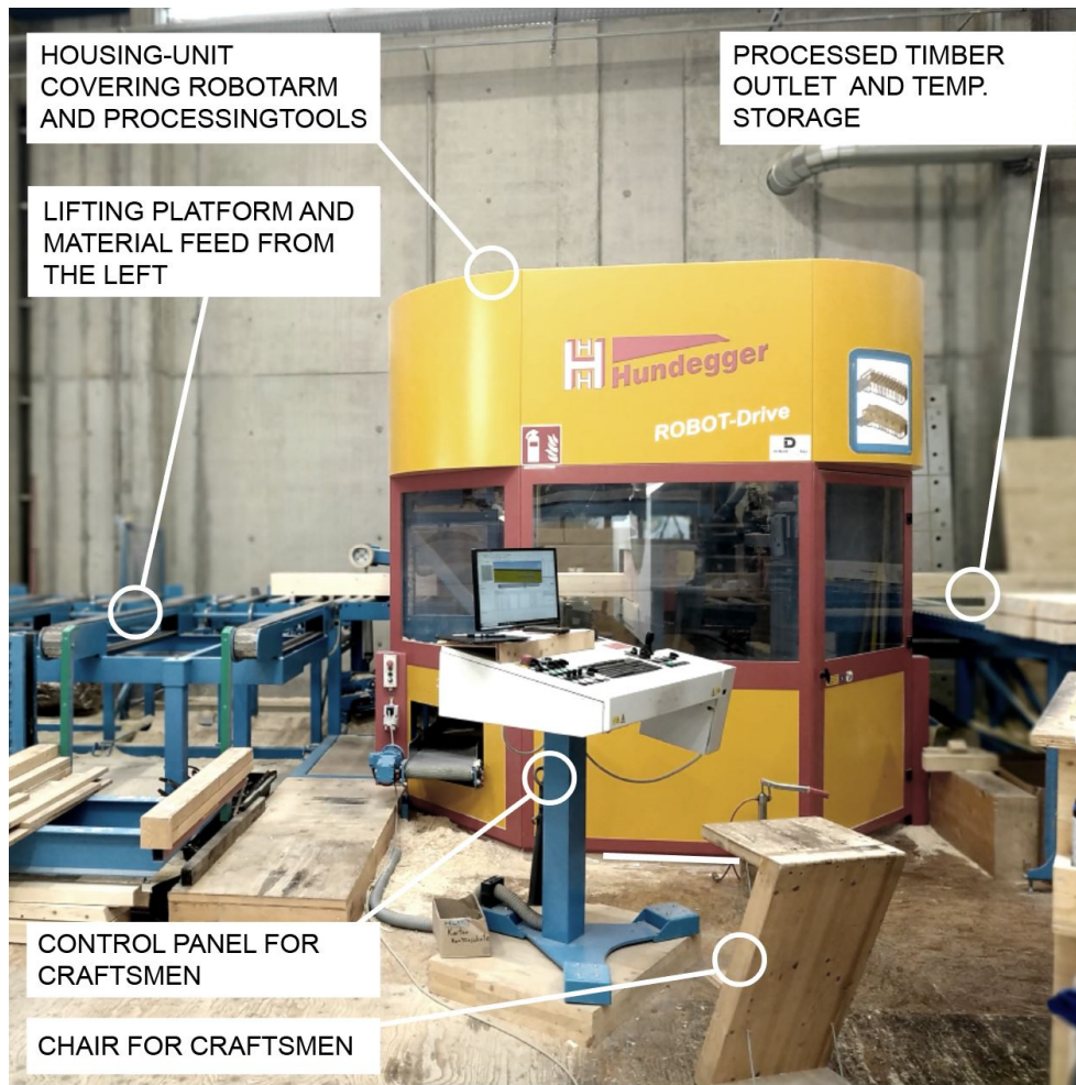
Figure 8. The joinery robot's milling machines are located under the yellow housing. Material is fed in from the left and then expelled on the right.
