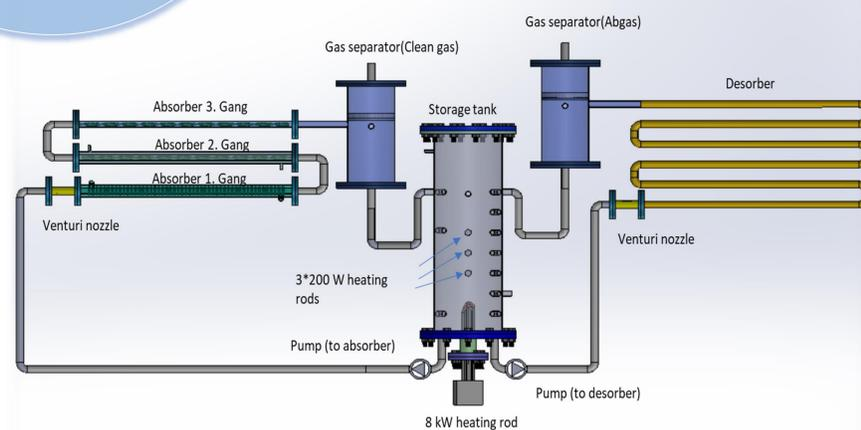
Fig. 6: Construction of pilot-scale continuously operating plant
