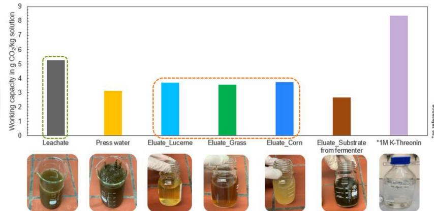
Fig. 3: Working capacity of different solutions from lab-scale batch experiment
