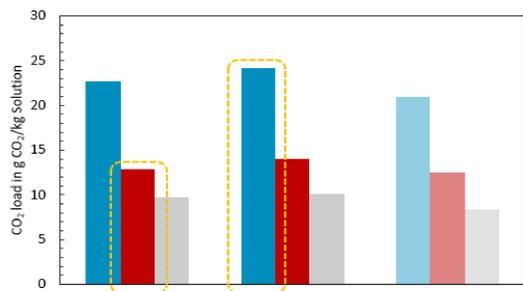
Fig. 5: CO<sub>2</sub> loads of the solution after absorption and regeneration from pilot-scale batch experiment
