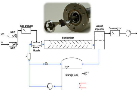
Fig. 4: Experimental set-up for pilot-scale batch operation
