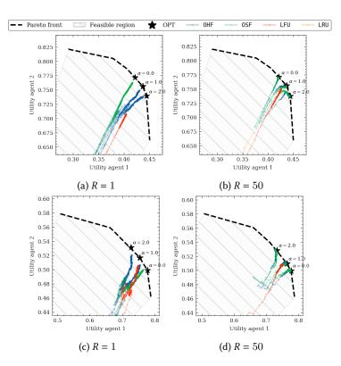
Fig. 7. Time-averaged utilities of policies OHF, OSF, LRU, and LFU under CYCLE topology. Subfigures (a)–(b) are obtained under retrieval cost  $w_{(1,3)} = 3.5$  for agent 1's query node. Subfigures (c)–(d) are obtained when agent 2's query node generates *Stationary trace* ( $\sigma = 0.6$ ). Markers correspond to iterations in {100, 200, ..., 10<sup>4</sup>}.
