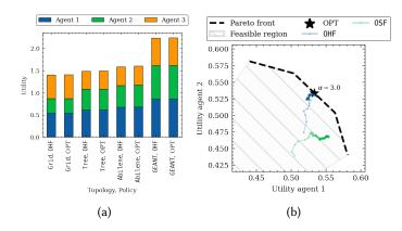
Fig. 11. Subfigure (a) provides the average utility of OHF and fairness benchmark under network topologies TREE, GRID, ABILENE, GEANT, *Stationary* trace ( $\sigma \in \{0.6, 0.8, 1.2\}$ ), and  $\alpha = 3$ . Subfigure (b) provides the time-averaged utilities obtained for OHF, OSF and batch size R = 50,  $t \in \mathcal{T}$ , under network topology Tree (a) and *Non-stationary* trace. The markers represent the iterations in the set  $\{100, 200, \dots, 10^4\}$ .
