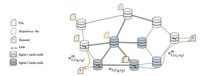
Fig. 4. System model: a network comprised of a set of caching nodes *C*. A request arrives at a cache node  $c \in C$ , it can be partially served locally, and if needed, forwarded along the shortest retrieval path to another node to retrieve the remaining part of the file; a utility is incurred by the cache owner  $i \in I$ . A set of permanently allocated files are spread across the network guaranteeing requests can always be served.
