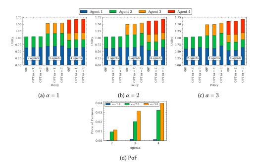
Fig. 9. Subfigures (a)–(c) provide the average utility for different agents obtained by OHF, fairness benchmark (OPT for  $\alpha \neq 0$ ), and utilitarian benchmark (OPT for  $\alpha = 0$ ); and Subfigure (d) provides the PoF for  $\alpha \in \{0, 1, 2, 3\}$  under an increasing number of agents in  $\{2, 3, 4\}$  and TREE 1–3 network topology.
