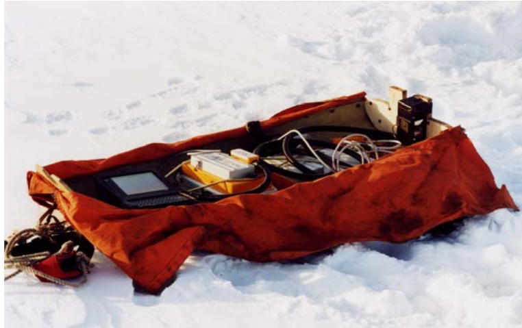
Figure 15. RAMAC GPR mounted into a little Pulka.
