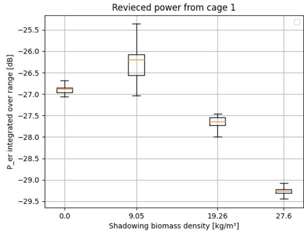
Fig. 6. Average received power from cage 1 (topmost cage). Cage biomass density referees to the shadowing biomass i.e cage 2
