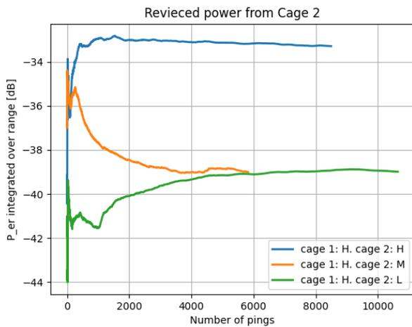
Fig. 9. Biomass number over pings from the Greek data. this plot shows the signal from the bottom cage over various biomass
