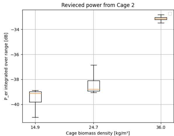
Fig. 11. Average received power from cage 2 (bottom cage). Cage biomass density referees to the shadowing biomass i.e cage 2
