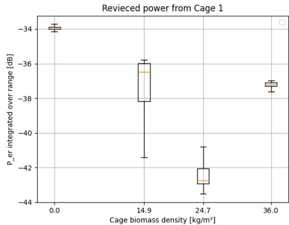
Fig. 10. Average received power from cage 1 (topmost cage). Cage biomass density referees to the shadowing biomass i.e cage 2
