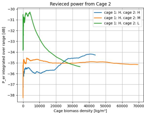
Fig. 5. Biomass number over pings from the Norwegian data. this plot shows the signal from the bottom cage over various biomass densities
