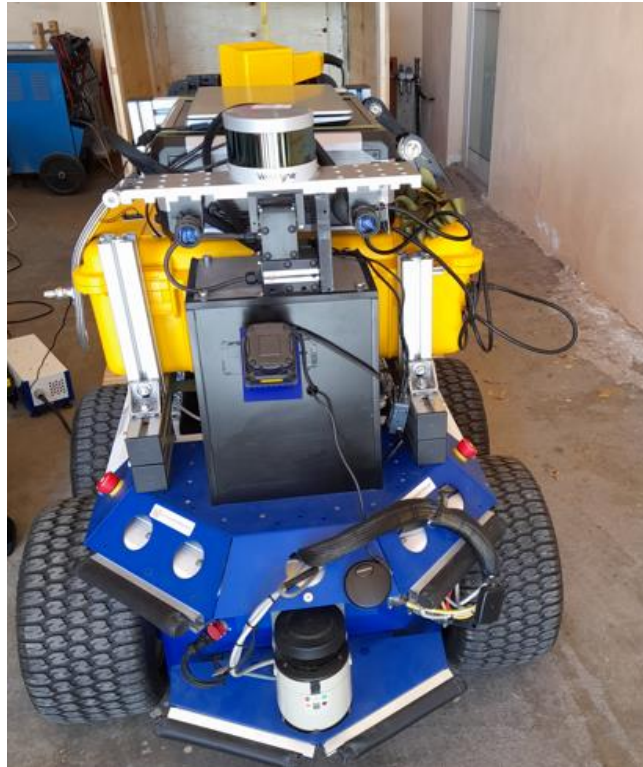
Figure 28: Final configuration of the SeekurJr DFKI robot after hardware integration of the RESCUE-MIMS device and its battery by NTUA
