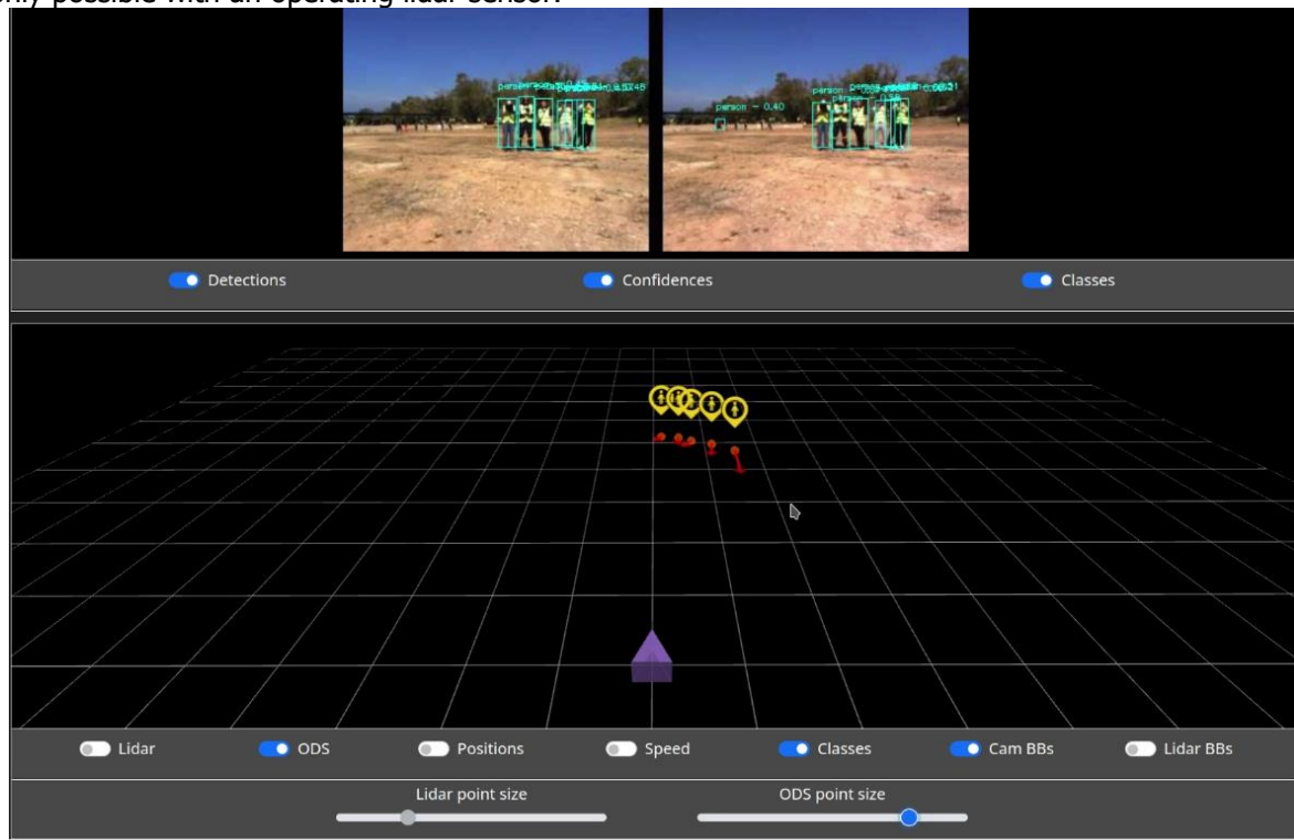
Figure 39: Web viewer screenshot of person detection after the latest upgrade. Yellow circles clearly mark persons. In the lower part, the visual show does not include LiDAR contribution.
