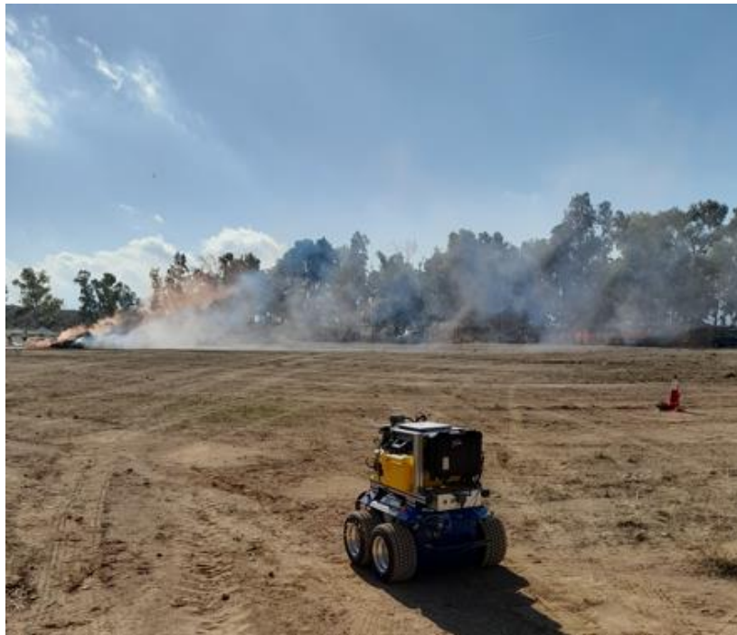
Figure 30: The RESCUE-MIMS (NTUA) on-board SeekurJr robot (DFKI) operating in UC4 simulated industrial fire scenario at Corinth field area, Greece
