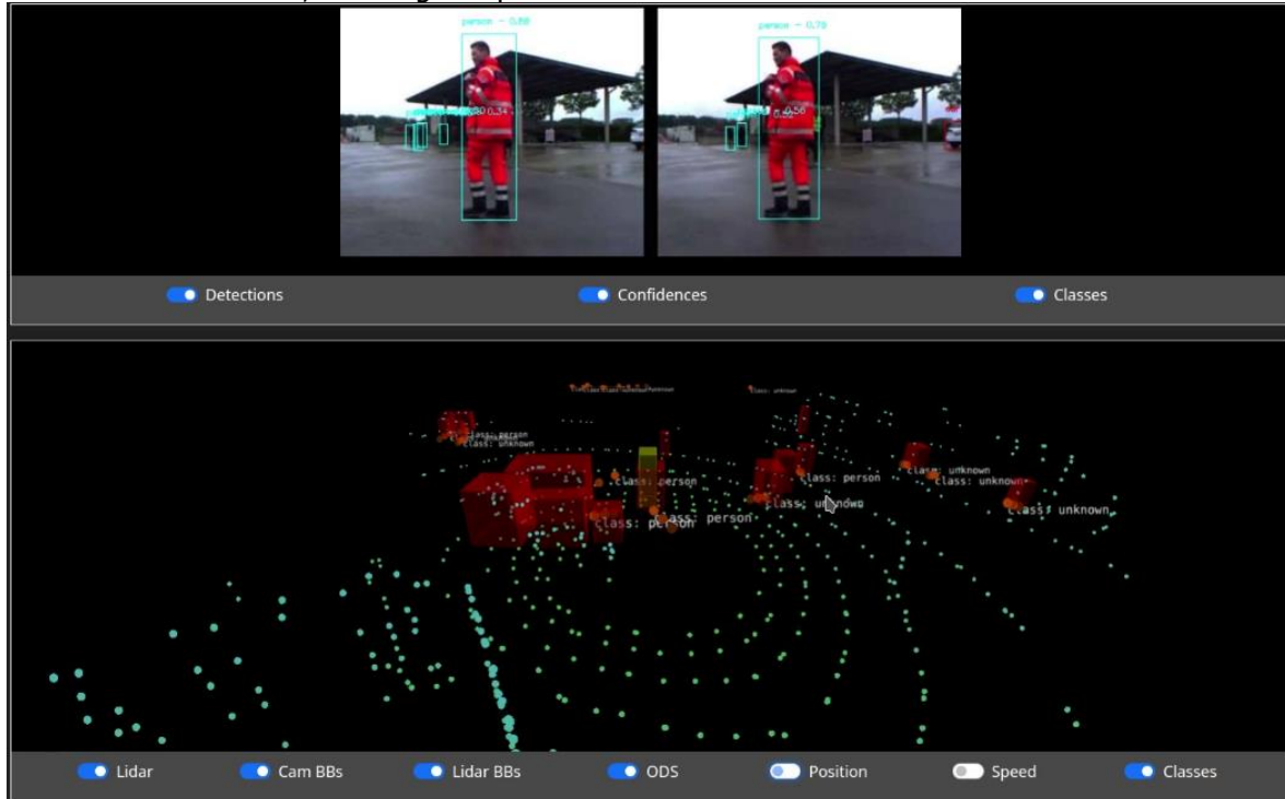
Figure 36: Web viewer screenshot of person detection. In the lower part the visual show of contributions from several sensors.
