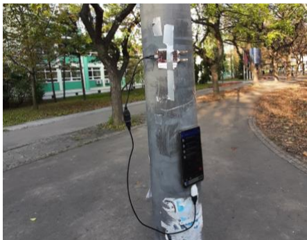
Figure 25. Recording setup: Audiohub - Nano with two microphones connected by USB connection to a mobile phone
