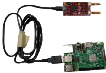
Figure 22. MemS microphones connected with the Raspberry Pi
