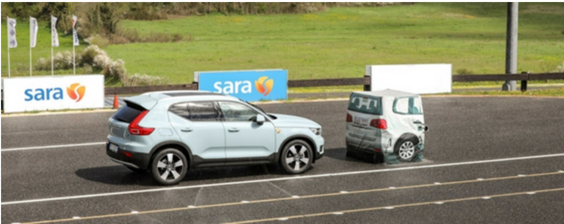
Figure 25 Emergency braking test with a vehicle silhouette
