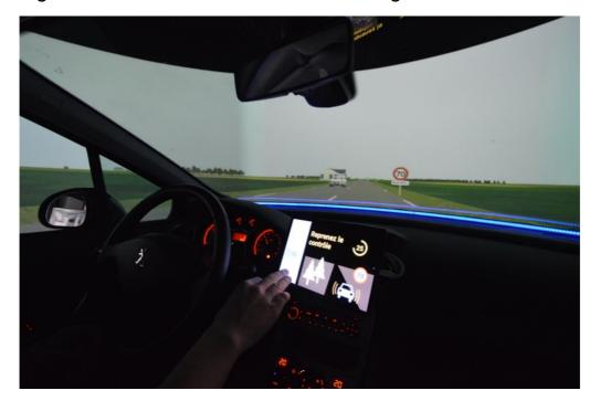
Figure 5 HMI embedded within the driving simulator
