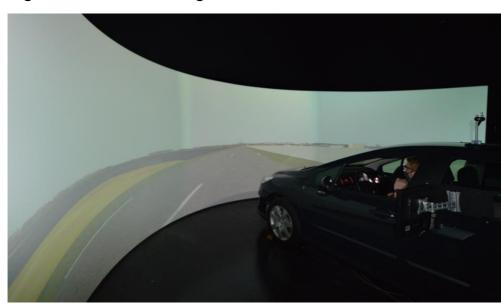
Figure 4 UBFC's driving simulator
