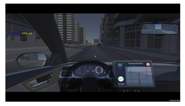
The GPS navigation system can be seen in the previous figures. A red line indicates the desired route, along with a dot which indicates the position of the car with respect to the route and surrounding streets. The interface
