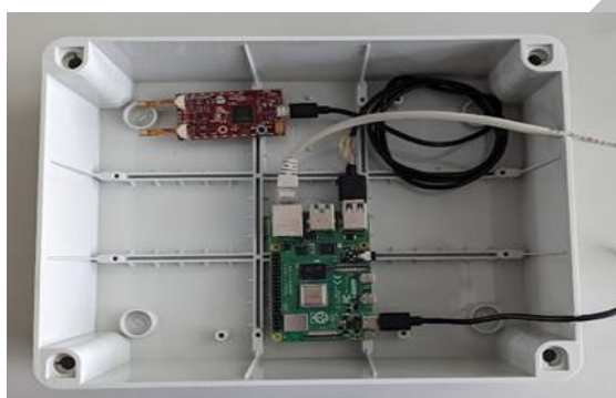
Figure 16: The "audio device" currently deployed in the MT3 use case. MEMS microphones are connected to the NanoHub board by IFAG (red one). The green board is the Raspberry PI. The reset board is not visible here
