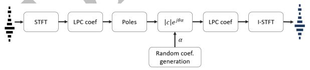
Figure 6: Processing pipeline of the approach based on McAdams coefficients
