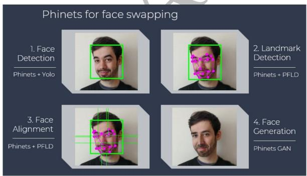
Figure 9: Processing steps of the MCU-based face-swapping component
