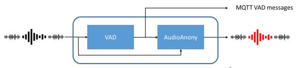
Figure 3: Block diagram of the joint VAD+AudioAnony component
