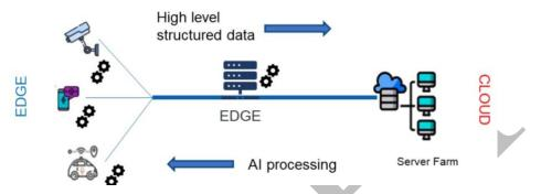
Figure 12: Edge-Fog processing: AI algorithms are deployed on the edge devices or on the fog, while only structured information is transferred to the cloud
