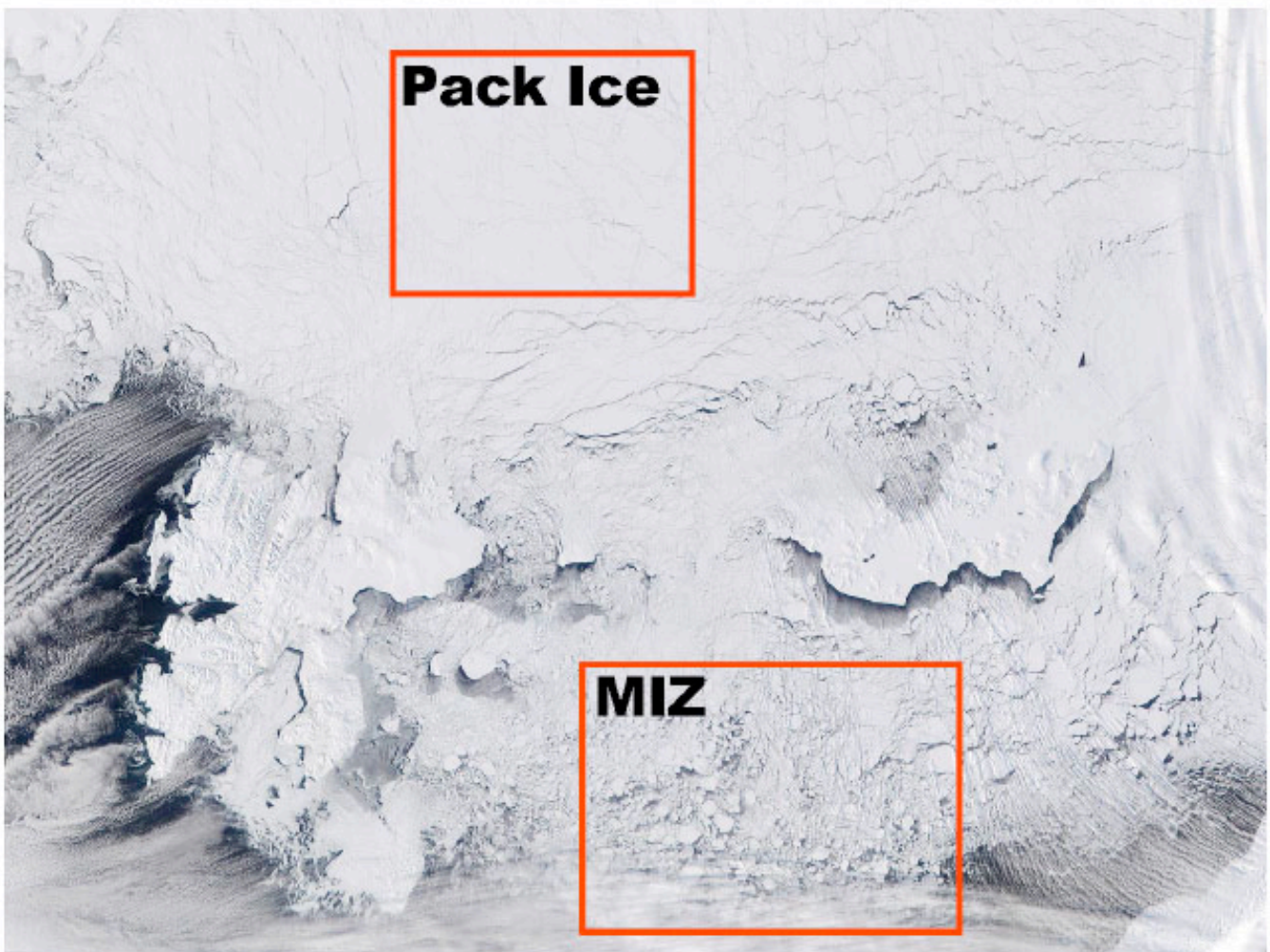
Figure 4.2. Illustration of a wintertime situation near Svalbard in 2003. The properties of the central ice pack and the MIZ are illustrated, with the MIZ consisting of a more broken-up ice field and a more granular appearance. (Image courtesy of NASA)
