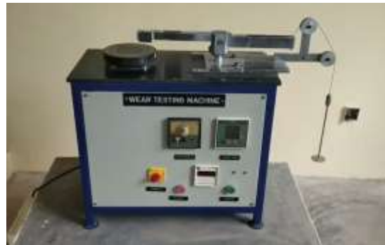
Fig 2 wear test machine
