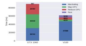
Figure 12: Execution Breakdown of Logistic Regression on two GPUs, a GTX 1060 (left bar) and a Tesla V100 (right bar).
