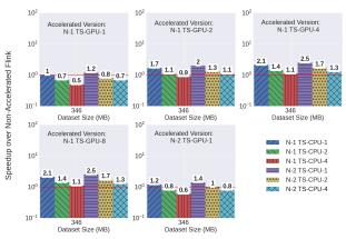
Figure 17: IoT Analytics: Performance of the Proposed System against Baseline Flink. The higher, the better.
