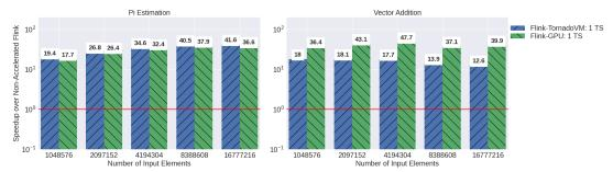
Figure 13: Performance of the Proposed System and Flink-GPU against Baseline Flink for Pi Estimation (left) and Vector Addition (right). The higher, the better.
