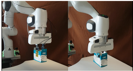
Fig. 2. Grasping of opened medicine box. On the left, the EAD gripper successfully grasp the box without altering its geometry. On the right, the classic parallel-jaw gripper deforms the box during grasping.
