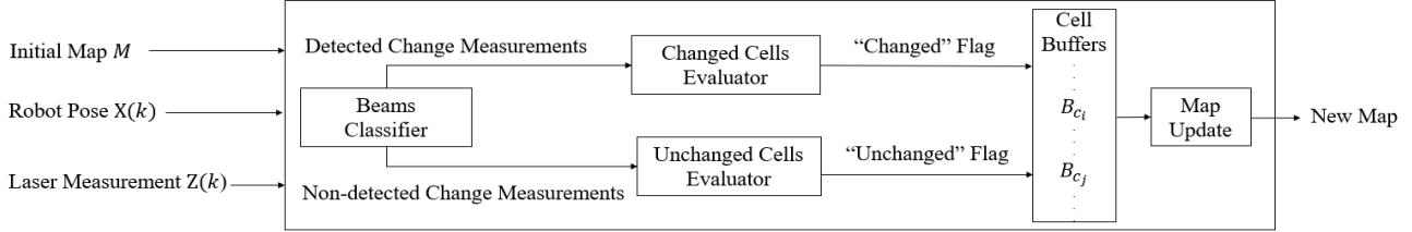
Fig. 1: System Overview: Measurements are classified as “detected change” or “non-detected change” w.r.t. the initial map by the *Beam Classifier*. Based on this classification, a rolling buffer  $B_{c_j}$  of each cell  $c_j$  is filled by the *Changed Cells Evaluator* and the *Unchanged Cells Evaluator* respectively through “changed” and “unchanged” flags. Finally, the state of the cells is updated if the number of “changed” flags in the buffer is higher than a given threshold.
