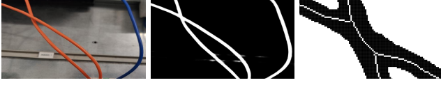
Fig. 2: Input image with background segmentation, result and generated skeleton zoomed at the intersections area.
