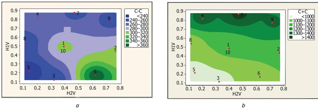
Fig. 4. Distribution of combinations of factors (setting points 1–10) in a 2D map in the coordinate  $H1/H2$ , which overlaps with the contour graphs of the response associated with experimental scheme 1, where the following factors were used:  $c$  – concentration of salt water solution (%) and  $s$  – distance to the ultrasonic unit (cm):  $a$  – response surface of the concentration of negative air ions ( $C^-$ );  $b$  – positive air ion concentration response surface ( $C^+$ )
