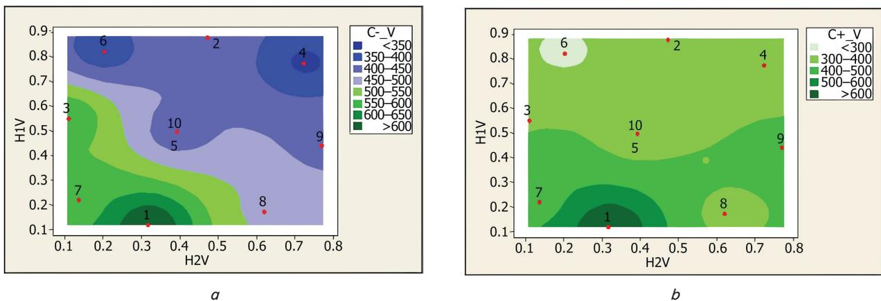
Fig. 5. Distribution of combinations of factors (setting points 1–10) in a 2D map in H1/H2 coordinates overlapping with a contour response graph related to experimental scheme 2, where the following factors were used:  $v$  – airflow rate (m/s) and  $s$  – distance to the ultrasonic unit (cm): *a* – response surface of the concentration of negative air ions ( $C^-$ ); *b* – positive air ion concentration response surface ( $C^+$ )
