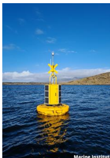
Figure 14. The Mobilis DB2000 data buoy deployed at the Marine Institute, Lehanagh Pool, Ireland.
