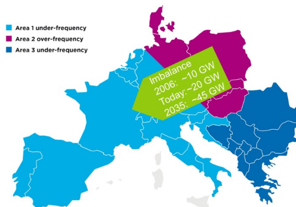
Fig. 1: Potential development of power imbalances in the event of a system split (e.g. on 4 th Nov 2006)
