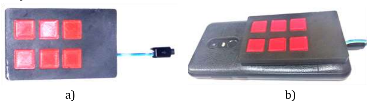
Fig. 2. Proposed external USB Braille keyboard for smartphones: a) The real view of the proposed keyboard; b) The state of the proposed keyboard connected to the smartphone (Android)
