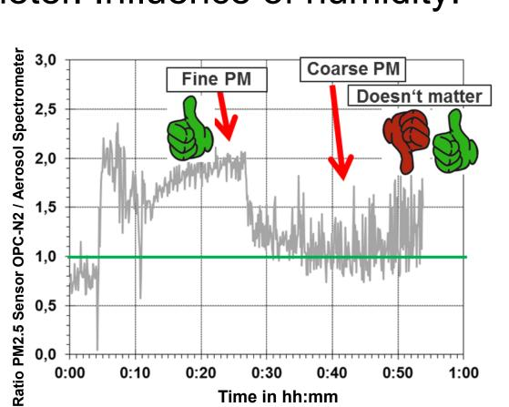
OPC-N2 is very suitable for making measurements, but need to be corrected by
