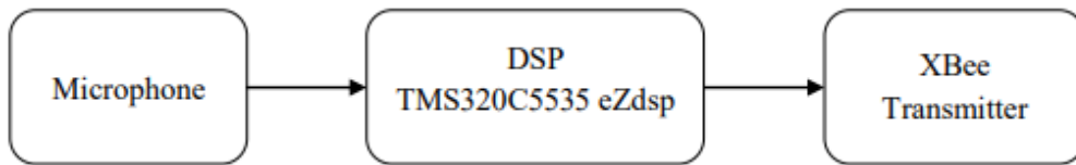
Figure 2. Block diagram of the sound processing part.
