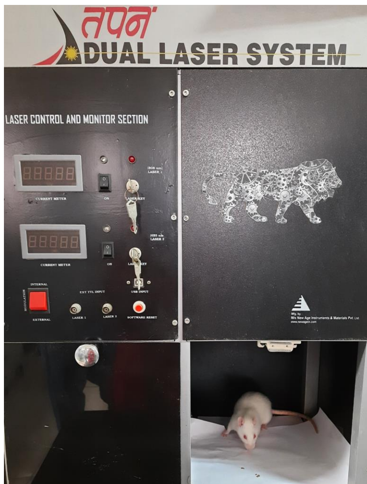
Figure 1: Positioning of the rat during photobiomodulation therapy with 808nm/655nm diode laser applied alone and on LPS treated rats
