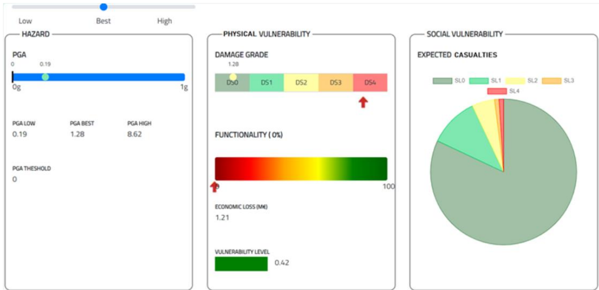
Figure 21 Dashboard for RRE - impacted infrastructure (detail)
