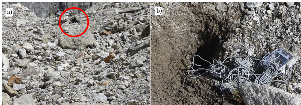
Figure 3.3: a) Surrounding area of an example pit (SBP5) as shown here. A red circle indicated a person sitting near the pit. b) Pit SBP5 dug on Satopanth Glacier for temperature measurement. The temperature sensors were inserted on the pit wall, which was connected to the data logger on the surface.
