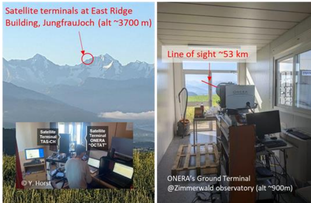
Figure 4. Setting of the VERTIGO outdoor demonstration. Both optical terminals were coupled to various telecom terminal provided by ETHZ and TAS, allowing to test a large panel of modulation formats over a wide range of turbulence conditions and SNRs.
