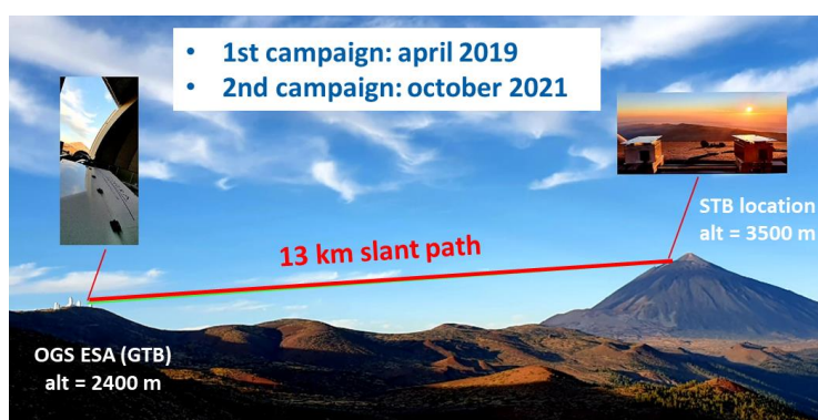
Figure 1. Summary of the FEEDELIO experiment (© G. Artaud). The ground station emulator (GTB) is inside the ESA OGS, while the satellite emulator (STB) is in Teide cable car station.
